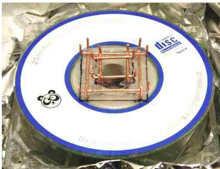
Figure E-1. Single-speed spin coater. Copper wire substrate holders visible on top.
