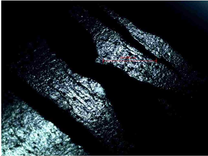
Figure 37: Image of side cracks 4.8 mol% Zr (U,Zr)O 2 pellet using Leica DM 2500P Microscope
