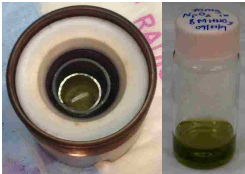
Figure 20: Neptunium dioxide and 8M \text{HNO}_3 loaded in a 23 mL Teflon autoclave, Resulting dark green solution after 72 hours digestion at 200 °C.
