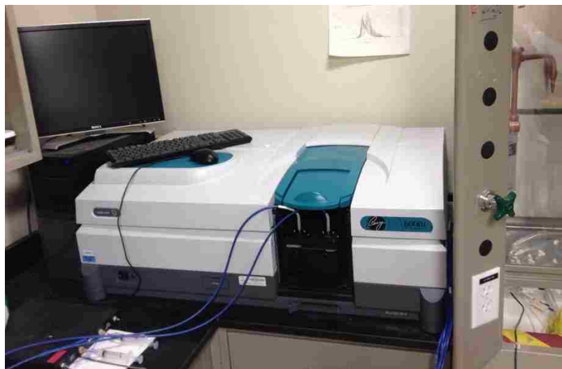
Figure 21 Cary 6000i UV-Visible with Ocean Optics 100cm liquid waveguide.
