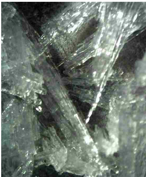
Figure 59 Sodium acetate crystals needles on which both the uranyl and americyl acetate crystals were grown.
