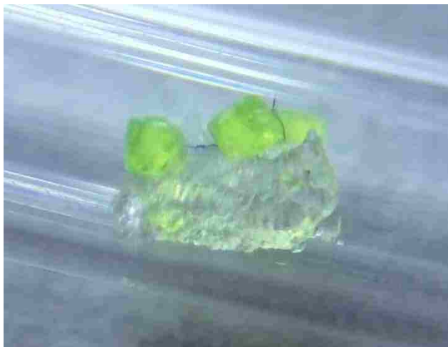
Figure 60 Close up showing the signature tetrahedral structure and yellow color of a cluster of sodium uranyl(VI) acetate crystal attached to sodium acetate crystals.
