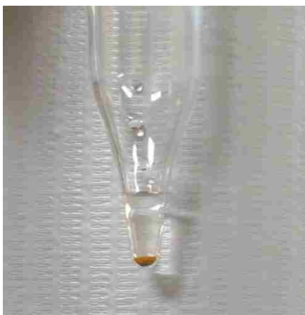
Figure 32 Oxidized Am(VI) sample ( 0.001\text{ M }^{243}\text{Am} in 1 M \text{HNO}_3 with \sim 2\text{ mg NaBiO}_3 excess solid on the bottom) prior to loading into the ANL/APS sample holder.
