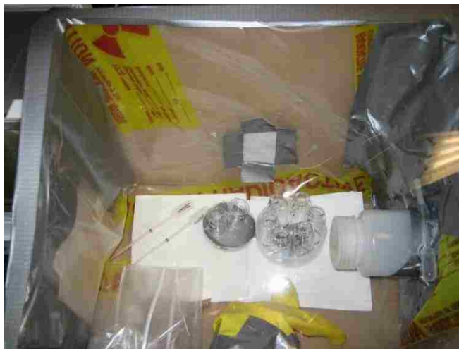
Figure 48 Secondary containment disposable glove box for sodium americyl(V) acetate crystal synthesis set inside a radiation hood.
