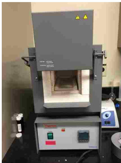
Figure 45 Thermo Scientific Thermolyne muffle furnace for fusion synthesis of \text{Li}_6\text{KBiO}_6 and \text{NaBa}_3\text{BiO}_6 crystals.
