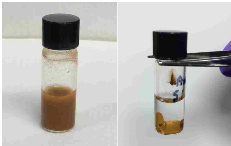
Figure 31 Oxidized ^{243}\text{Am} in 1 M \text{HNO}_3 solution with sodium bismuthate before and after centrifuging.
