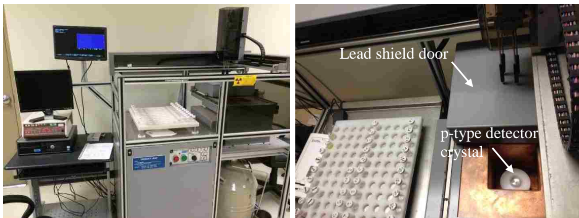
Figure 29 ORTEC ® GEM50P4-83 HPGe gamma ray detector with robotic sample changer.
