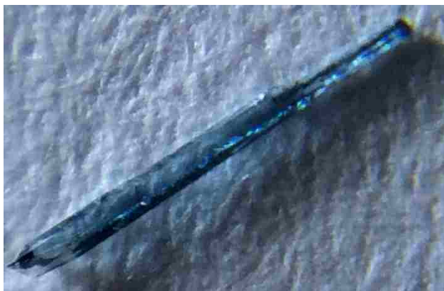
Figure 51 The \text{NaBa}_3\text{BiO}_6 \cdot \text{MnO} fusion produced blue-purple hexagonal needles with dimensions of \sim 0.5 - 1.0 mm on edge.
