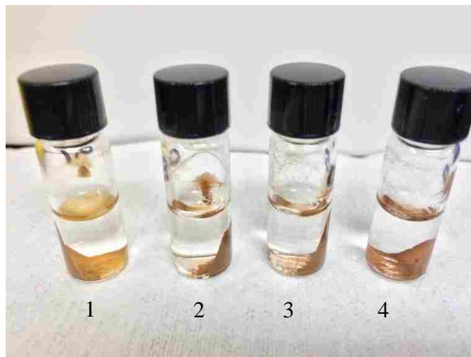
Figure 47 Excess sodium bismuthate in \text{HClO}_4 concentrations of: (1) 0.1 M, (2) 0.3 M, (3) 0.5 M, (4) 1.0 M. The liquid phase shows no coloration from the sodium bismuthate, however, the solid sodium bismuthate in concentrations above the 0.1 M \text{HClO}_4 has taken on a darker shade.
