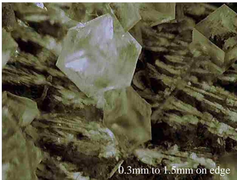
Figure 49 Pale yellow, cubic crystals of \text{Li}_3\text{KBiO}_6 which retain the Bi(V) oxidation state.
