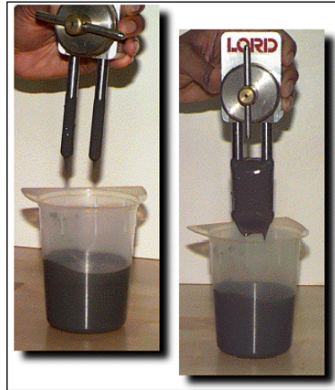
Figure 16. MR fluids. (a) Non-magnetic field (b) Applied to a magnetic field [7].
