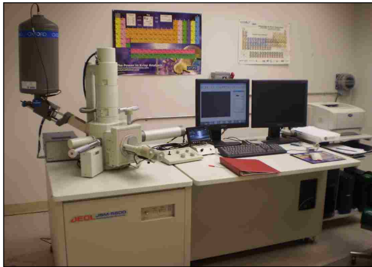
Figure 7 Scanning Electron Microscopy with EDS capabilities
