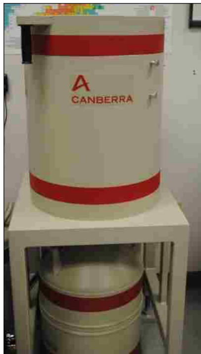
Figure 15 HPGe with liquid nitrogen Dewar
