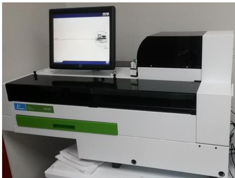
Figure 2.3 Wizard 2480 automated gamma counter
