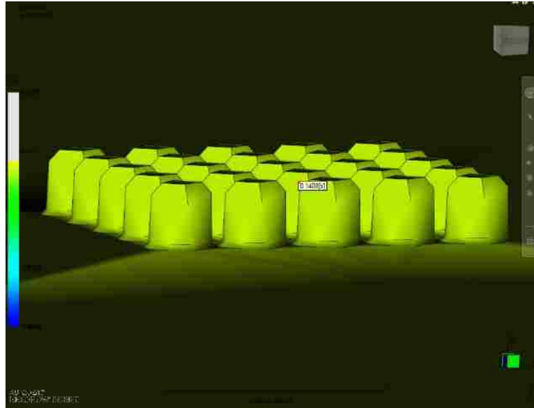
Figure 5-16: Micro-structured region filled at t=0.1408 sec.
