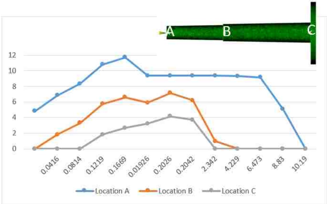
Figure 5-20: Pressure distribution during filling at different locations.
