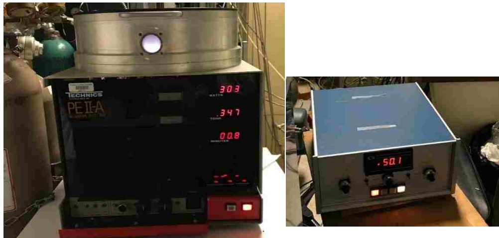
Figure 4-12: O 2 Plasma Ashing Machine.
