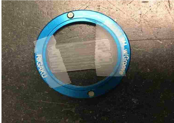
Figure 6-11: Sample attached to the XRD ring.
