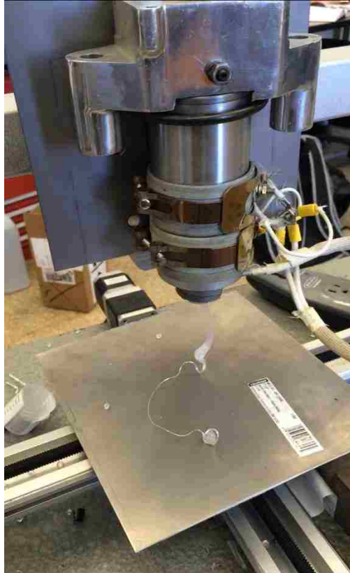
Figure 4-9: Polymer flowing out of the extruder after removing the nozzle.
