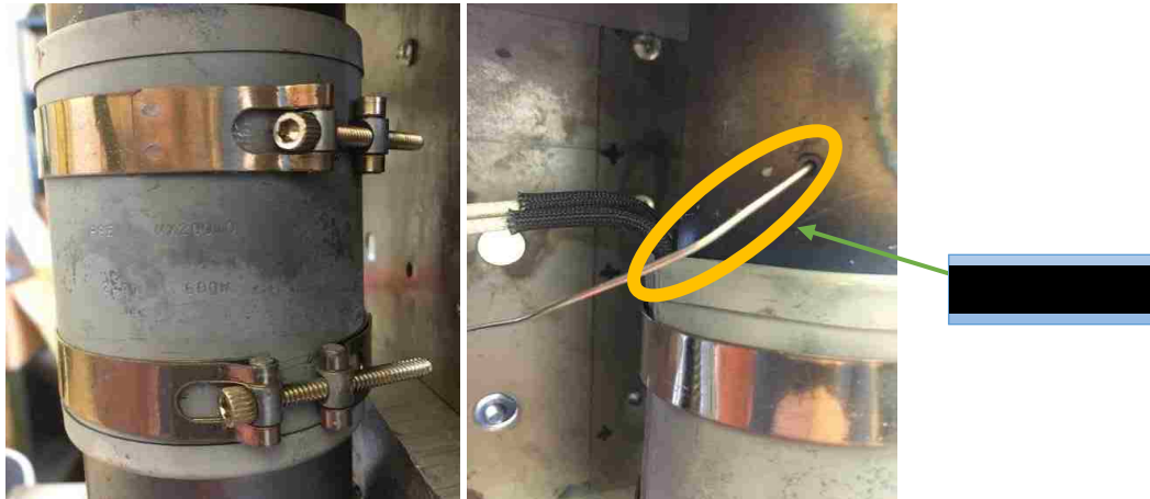
Figure 4-29: Band heater and J type thermocouple.
