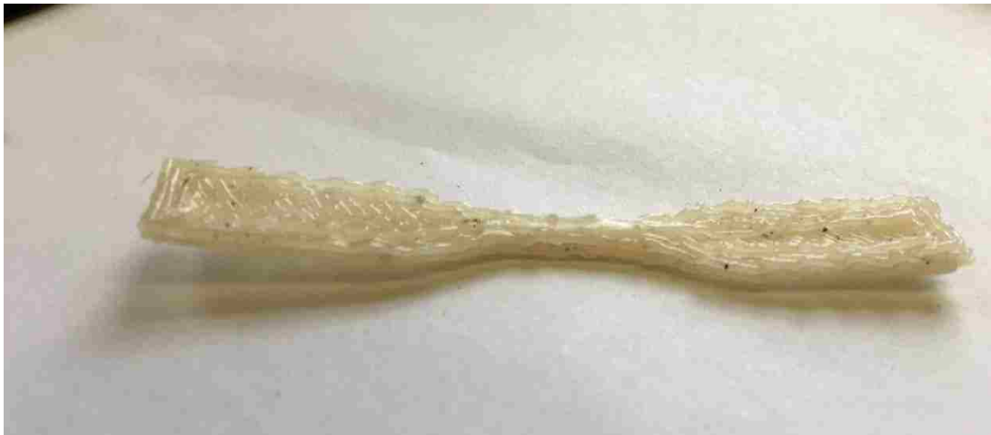
Figure 6-29: Part printed at stage temperature of 85°C, which caused it shrink.
