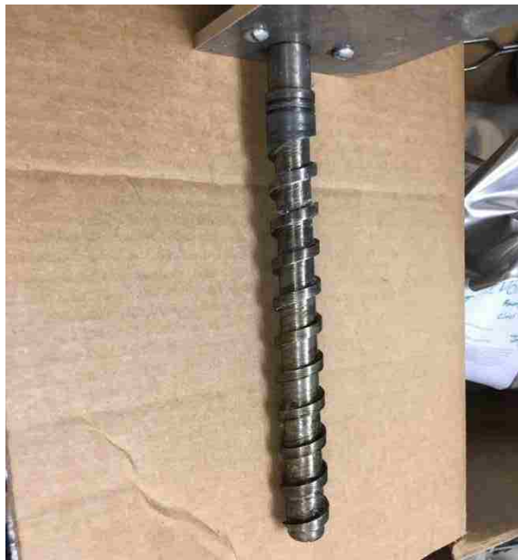
Figure 4-12: Screw extruder designed and developed for prototype 2.
