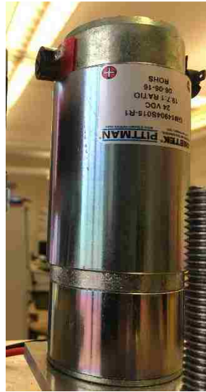
Figure 4-26: DC motor used for the screw extruder.
