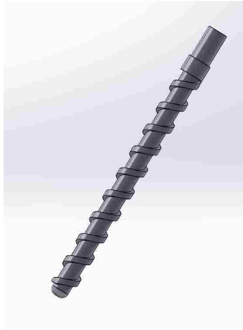
Figure 4-3: Extruder screw of Prototype 1
