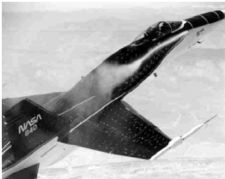
Figure 1.6: Smoke visualization of a vortex shed from the forebody of an aircraft. Vortex bursts upstream of the fin. Moses (1997)
