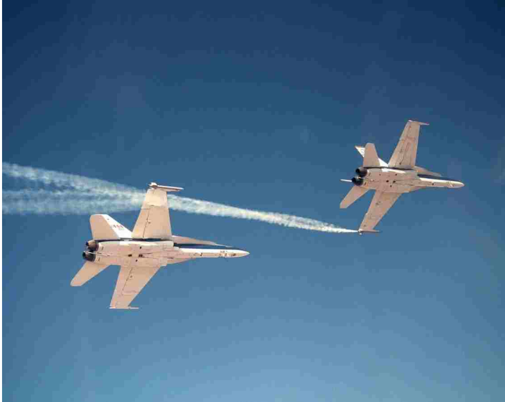
Figure 1.5: Smoke visualization of the impingement of a tip vortex shed from a leading aircraft onto the wing of a downstream aircraft. This image was taken as a part of NASA Dryden's Autonomous Formation Flight Project and features a pair of F/A-18s. Thomas (2001)
