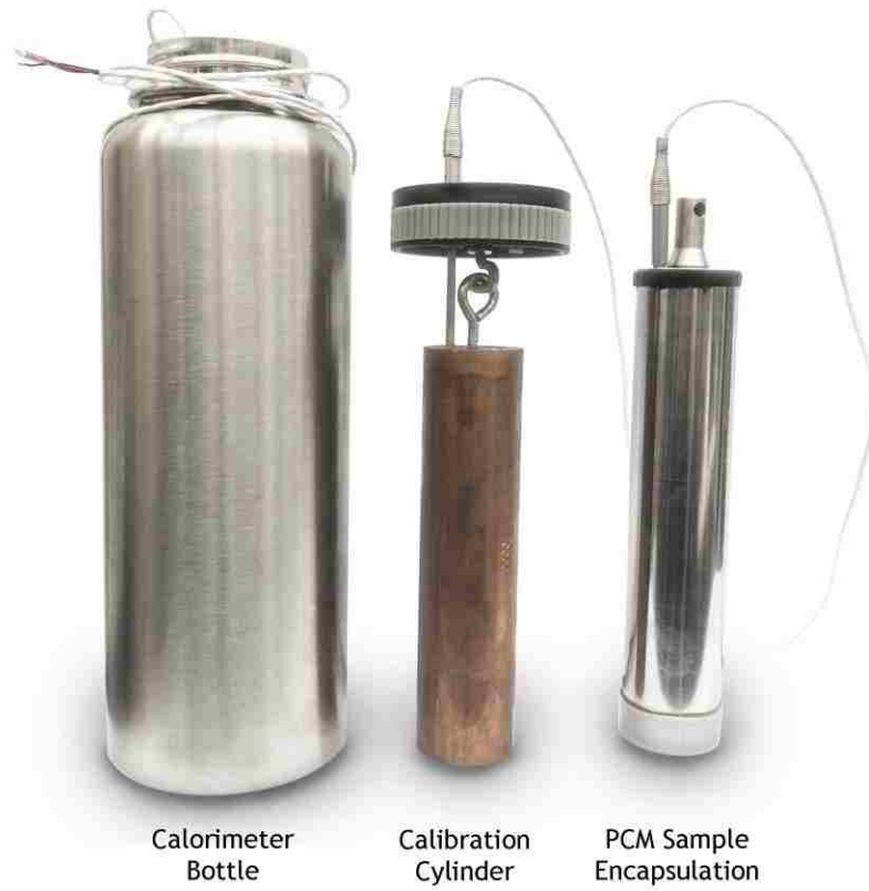
Figure 3.9: Calorimeter Bottle, Copper Calibration Cylinder, and PCM Sample Encapsulation
