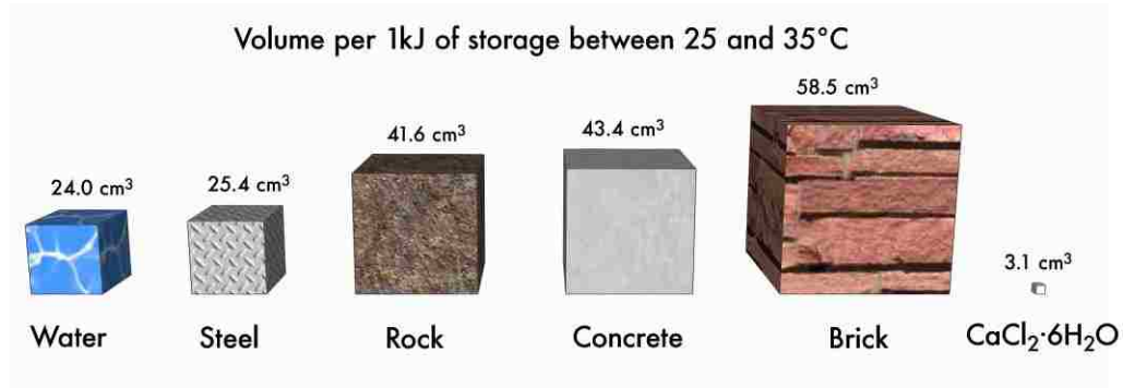
Figure 1.3: Volume of Material Required for 1 kJ of Storage Between 25 & 35°C
