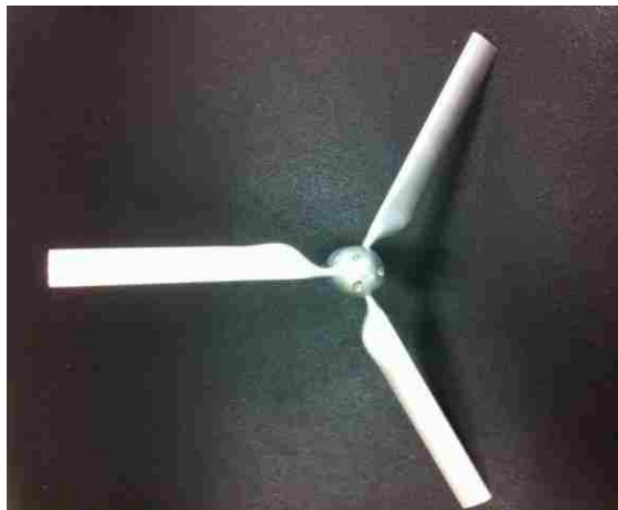
Figure 5.1: Photograph of turbine prototype used for current study [ R=0.14\text{m} ]
