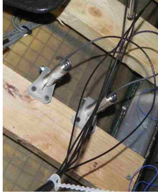
Figure 6-9 Static Load Test LVDTs
