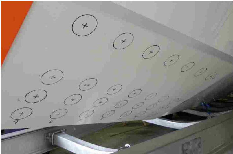
Figure 6-10 Static load test grid
