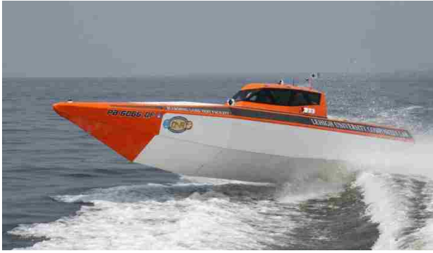
Figure 5-1: The Numerette slamming boat. The section behind the colored bow is the one presently studied
