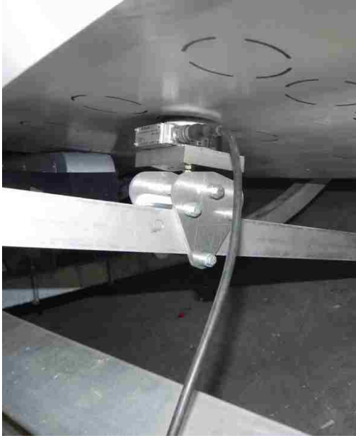
Figure 6-8 Static load test fixture
