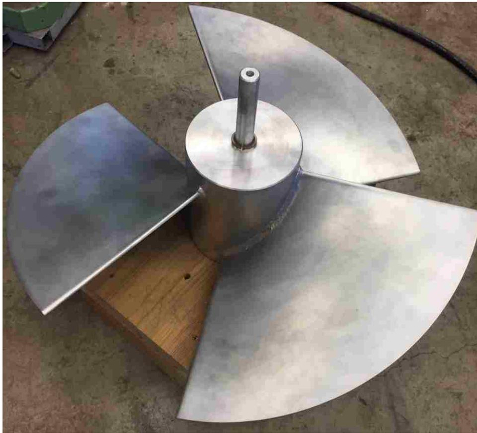
Figure 42. Final optimized blade design.
