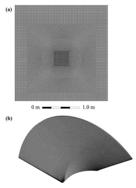
Figure 23. (a) Center of the computational domain for Fr = 0.70 and (b) grid along a singular turbine blade.
