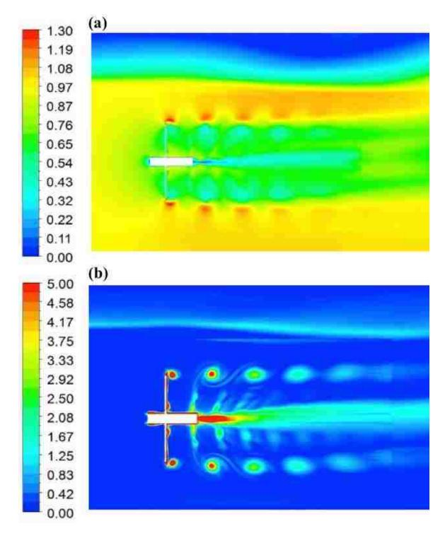
Figure 31. Normalized (a) velocity and (b) vorticity contours along the vertical meridional at a Froude number of 1.31 and a tip speed ratio of 1.86.
