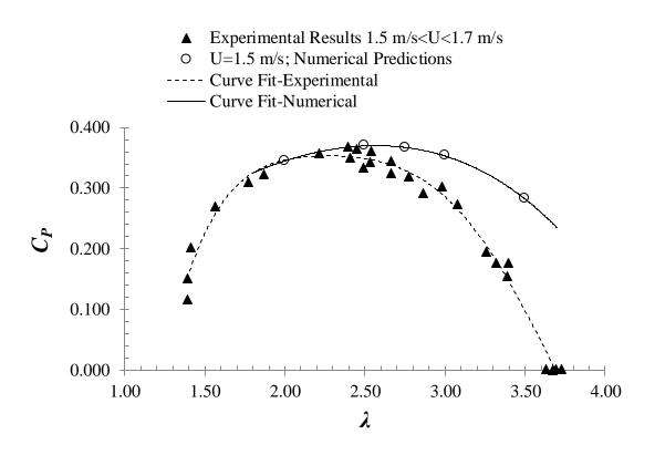
Figure 54. Power coefficient as a function of tip speed ratio for flow speeds ranging from
