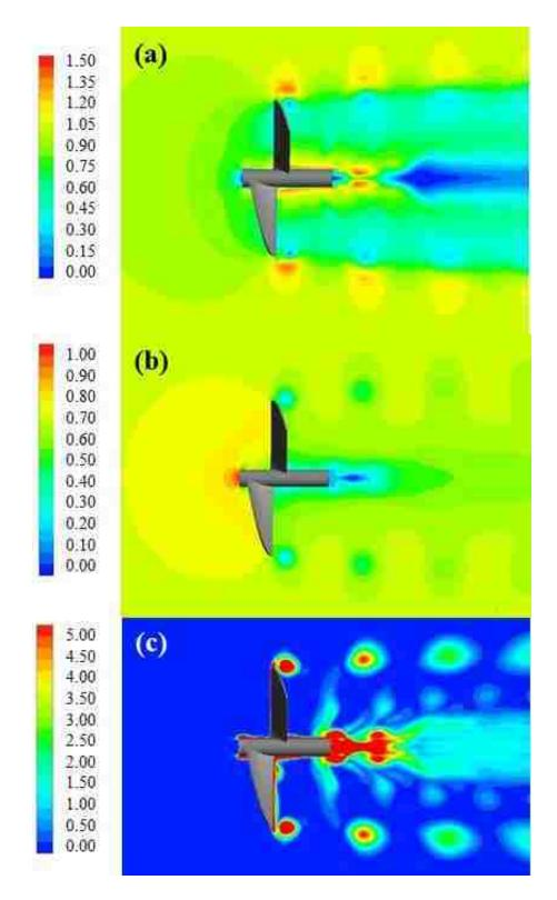
Figure 20. Steady-state turbine analysis with normalized (a) velocity, (b) pressure, and (c)
