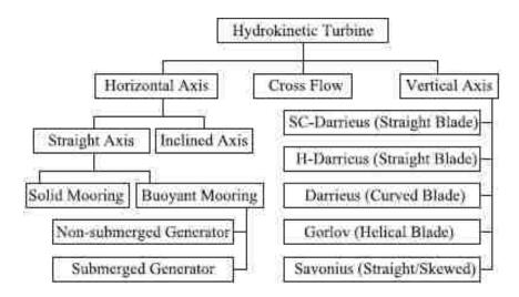
Figure 1. Hydrokinetic turbine classification [3]
