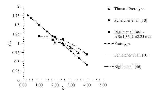
Figure 44. Coefficient of thrust as a function of tip speed ratio.
