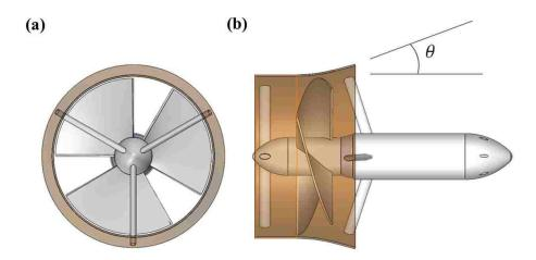
Figure 41. Prototype design (a) front view and (b) side view with diffuser implemented
