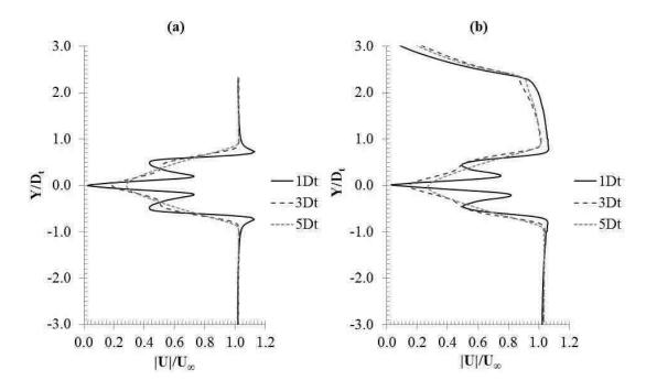
Figure 37. Profiles of the normalized streamwise component of the velocity for (a) single phase and (b) multiphase simulations at Fr = 0.71.
