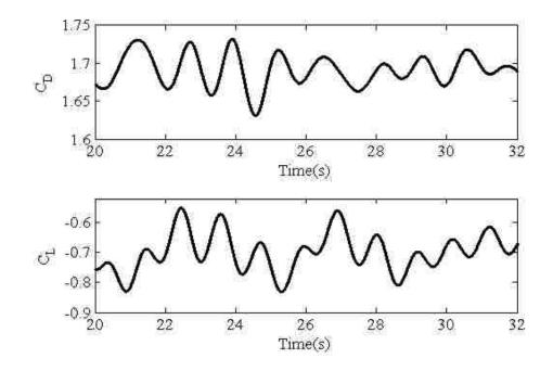
Figure 25. Values of coefficient of (a) drag and (b) lift with respect to flow time.
