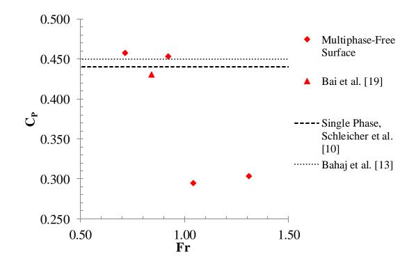
Figure 26. Power coefficient as a function of Fr [49].
