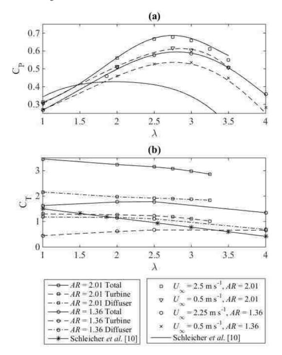
Figure 19. Predictions of (a) power coefficient and (b) thrust coefficient for turbinediffuser systems at area ratios of 1.31 and 2.01 for several freestream flows [45].
