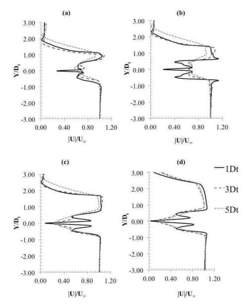
Figure 36. The profiles of the normalized streamwise component of the velocity for Fr of (a) 1.31, (b) 1.04, (c) 0.92, and (d) 0.71 at various locations downstream of the turbine. 86
