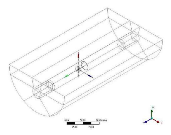
Figure 13. Computational domain used for DAHkT and individual hydrokinetic turbine modeling and optimization with flow moving from left to right.
