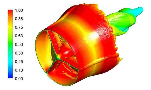
Figure 52. Normalized velocity contours along vorticity ropes at a normalized vorticity of 1.0. *Experimental Results*
