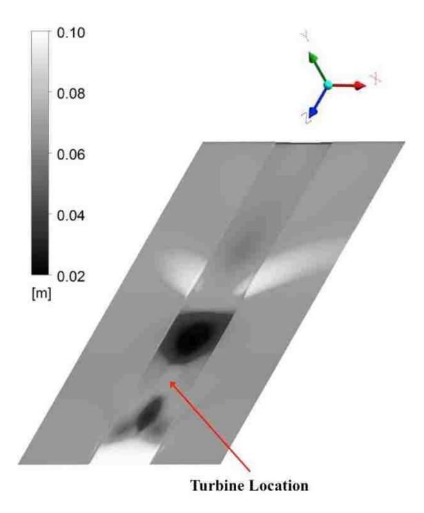
Figure 34. Isosurface of the free surface for cases of Fr=0.92.
