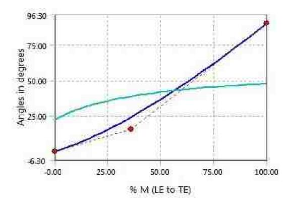
Figure 40. Blade curvature along the turbine mean line from the leading edge (LE) to trailing edge (TE) and relative blade angle (teal line).
