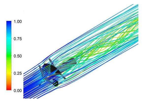
Figure 51. Normalized velocity along streamlines within the turbine domain.
