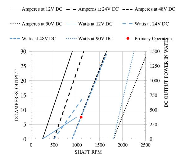
Figure 45. Shaft RPM vs DC output for chosen generator.
