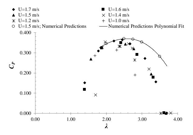
Figure 53. Power coefficient as a function of tip speed ratio at various flow speeds.
