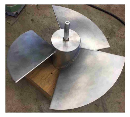
Figure 42. Final optimized blade design. 94
