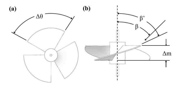
Figure 39. Propeller turbine blade (a) front view and (b) top view.
