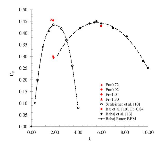
Figure 28. Power coefficient as a function of tip speed ratio for the traditional and propeller-based hydrokinetic turbine designs studied [9,12,18].
