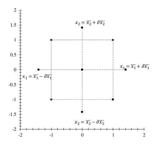
Figure 11. Example of a Central Composite Design for Two Independent Design Variables
