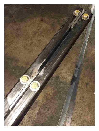
Figure 48. Welded support beam.
