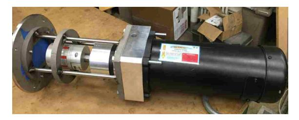
Figure 46. Generator assembly.
