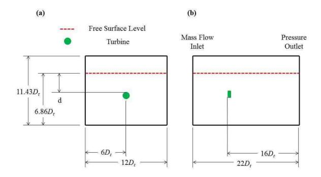
Figure 22. (a) Front view and (b) side view of the river domain with dimensions based on turbine diameter  $(D_t)$ .
