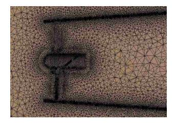
Figure 14. Tetrahedral mesh near turbine and diffuser walls 48
