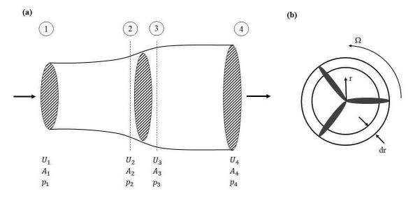
Figure 2. Stream tube through an (a) actuator disk and (b) schematic for rotating actuator disk
