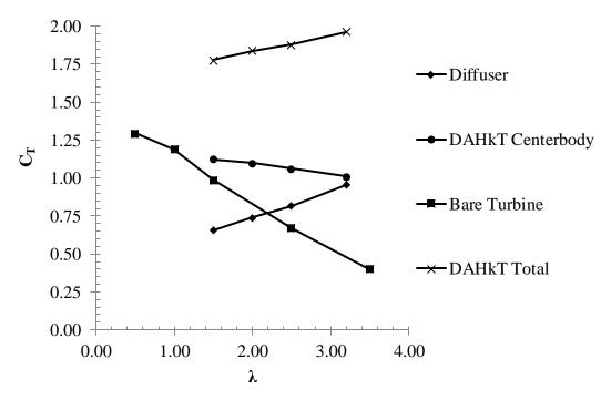
Figure 16. Thrust coefficient as a function of tip speed ratio.
