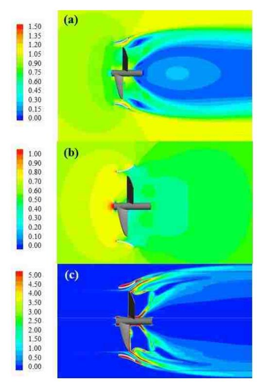
Figure 21. Steady-state turbine-diffuser analysis with normalized (a) velocity, (b) pressure, and (c) vorticity for AR=1.36.
