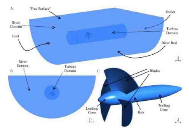
Figure 5. General boundary condition setup for RANS-CFD analysis [37].
