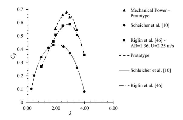
Figure 43. Power coefficient as a function of tip speed ratio from rapid CFD results.
