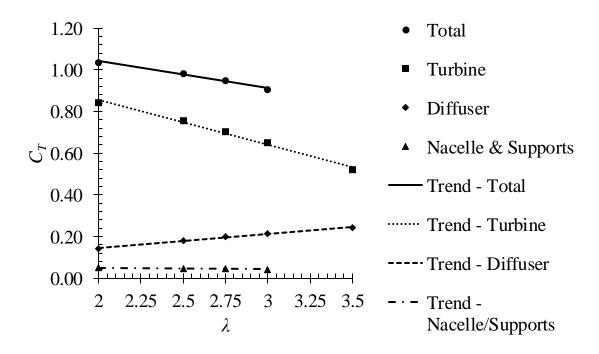
Figure 50. Prototype thrust coefficient predictions as a function of tip speed ratio.
