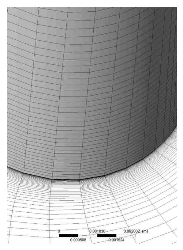
Figure 7. Boundary layer inflation along the blade and hub.
