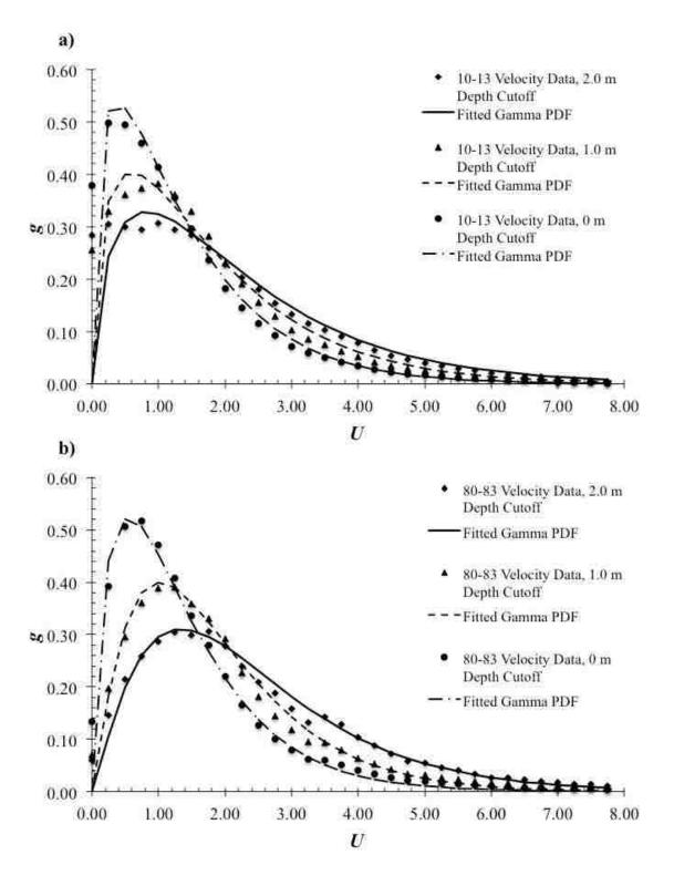
Figure 9. Gamma distribution function and measured results as a function of river velocity for data obtained from a) 2010 to 2013 and b) 1980 to 1983.
