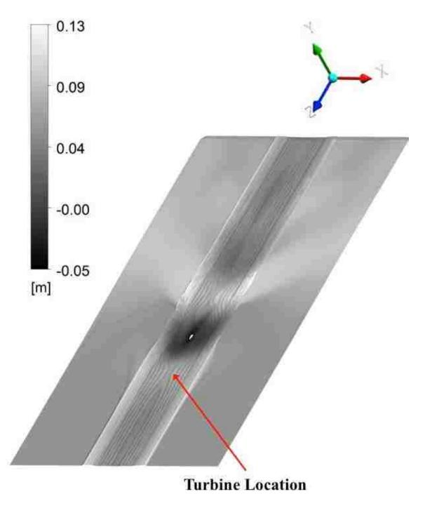
Figure 32. Isosurface of the free surface for cases of Fr=1.31.
