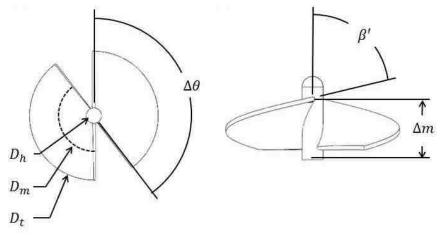
Figure 4. Preliminary turbine blade geometry.
