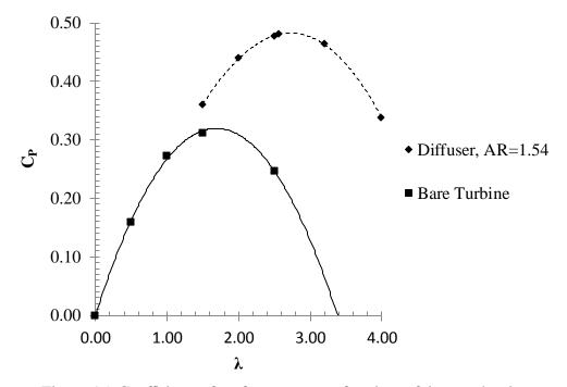
Figure 15. Coefficient of performance as a function of tip speed ratio.
