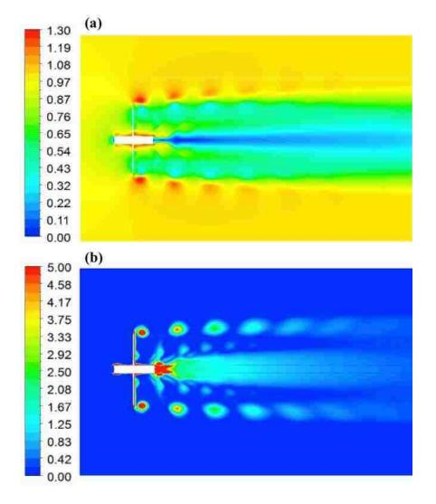
Figure 29. Normalized (a) velocity and (b) vorticity contours along the vertical meridional for single phase turbine operation in an infinite medium at a tip speed ratio of 1.86.
