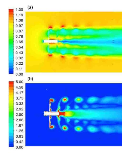
Figure 30. Normalized (a) velocity and (b) vorticity contours along the vertical meridional at a Froude number of 0.92 and a tip speed ratio of 1.86.
