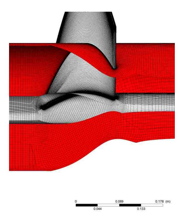
Figure 8. Grid structure along the meridional plane of the turbine design.
