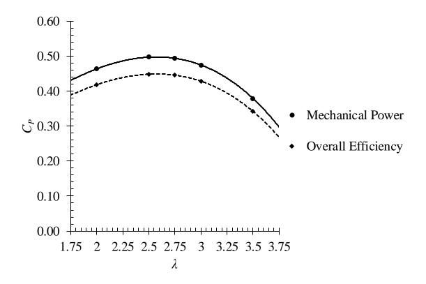
Figure 49. Prototype power coefficient predictions as a function of tip speed ratio.
