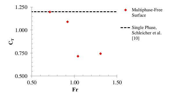
Figure 27. Thrust coefficient as a function of Fr [49].
