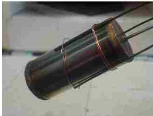
Figure 6. Thermocouples used to measure sample temperature secured with copper wire
