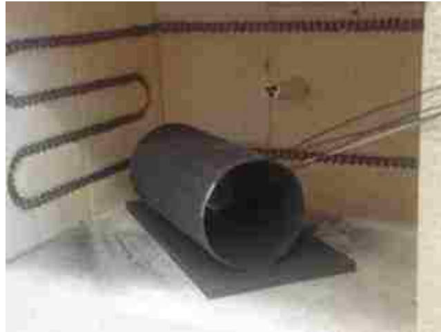
Figure 5. Sample placed in carbon steel cylinder during heating process
