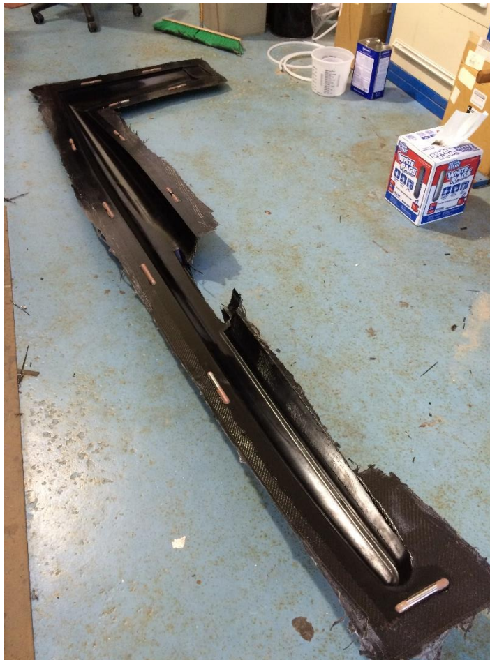
Figure 24. Finished Fuselage and Vertical Stabilizer Mold
