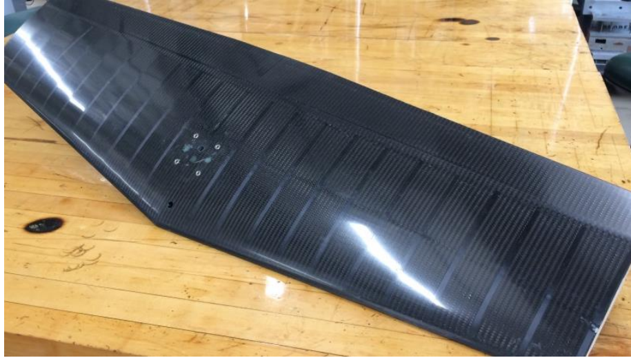
Figure 20. Finished Stabilizer and Elevator. This one has 5 mm wide strips of unidirectional carbon fiber placed on both sides of both skins; these increase cross sectional stiffness and buckling strength and in a sense work as lightweight ribs.
