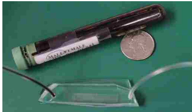
Figure 1-1 Patient blood is injected through a typical microfluidic device for CTC detection.
