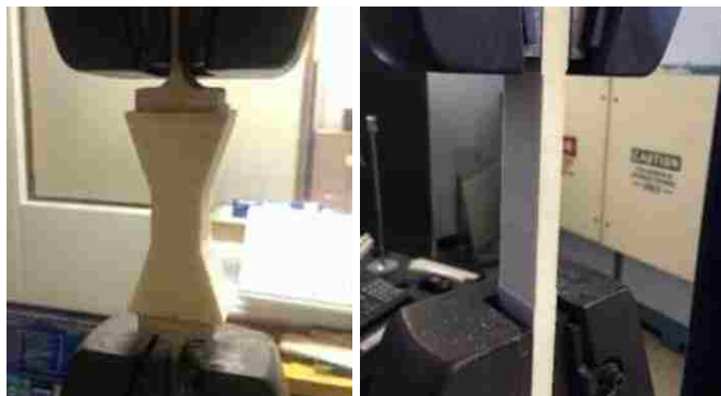
Figure 9. Polyisocyanurate foam characterization – uniaxial tensile test
