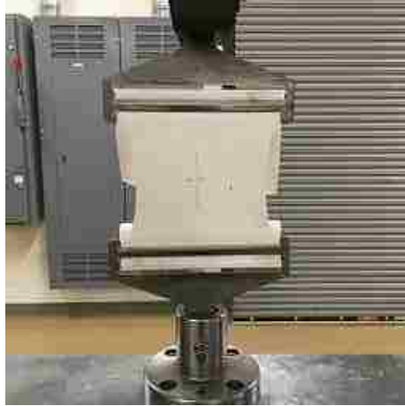
Figure 11. Strip-biaxial tension experiment set up for PVC/TPO membrane
