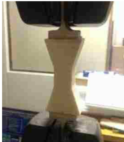
Figure 18. Uniaxial tension test to Polyisocyanurate foam dog-bone specimen
