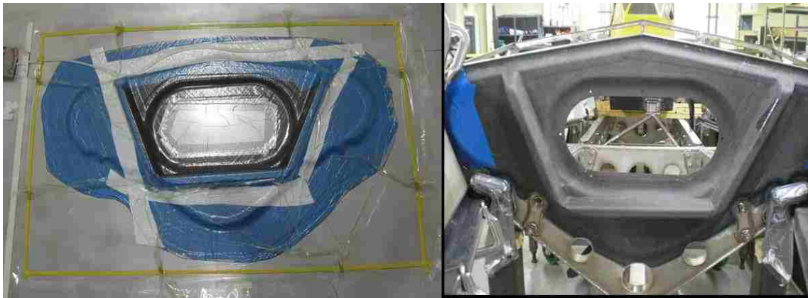
Figure 3-13: Manufacturing of the collision bulkhead panel and the panel installed
