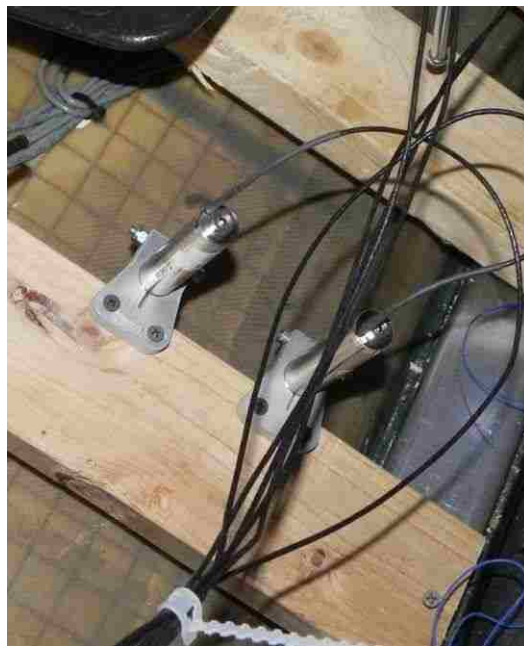
Figure 4-9: LVDTs mounted for static load tests
