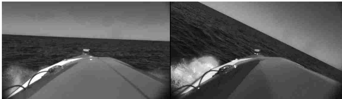
Figure 4-51: Neutral and High Roll Slamming Event Comparison
