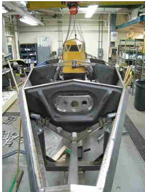
Figure 3-14: Assembly of bulkhead panels and side panels
