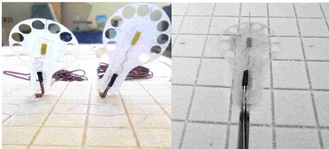
Figure 3-8: Strain gage paddles bonded to PVC foam core
