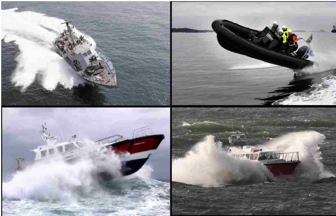
Figure 1: Demonstration of high-speed craft slamming events
