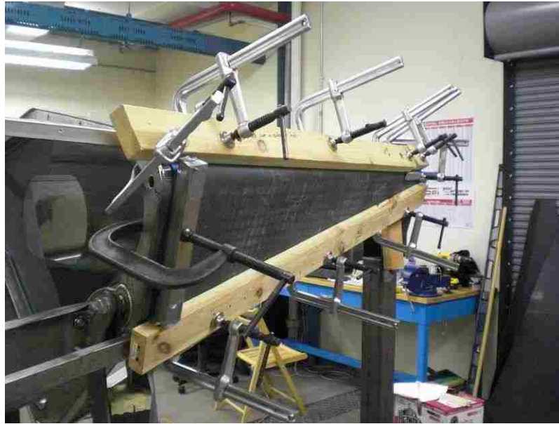
Figure 3-15: Bonding of a side panel
