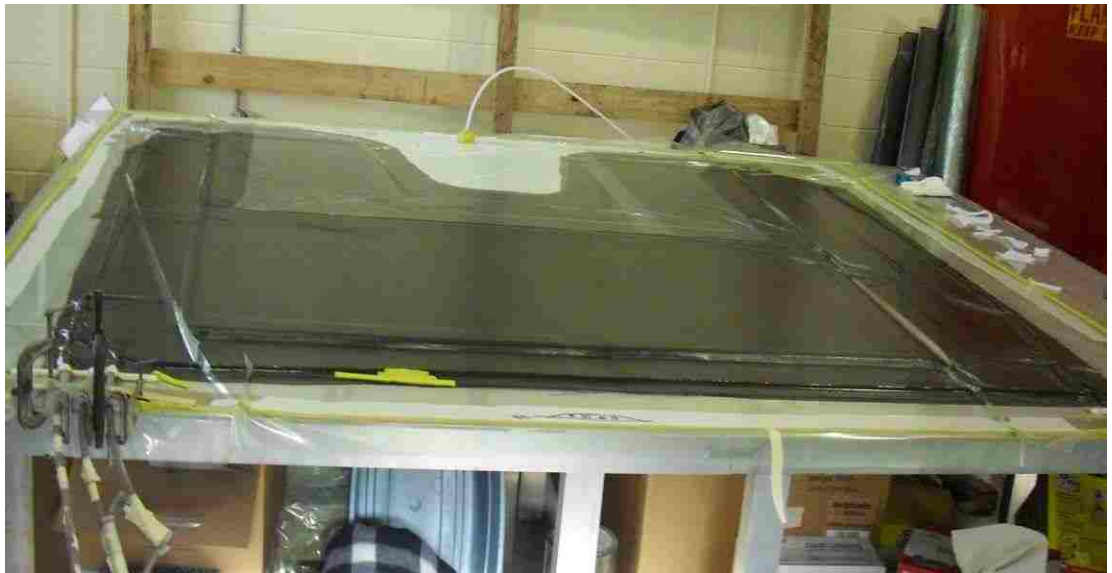
Figure 3-6: Manufacturing of the biggest composite panel on the boat.
