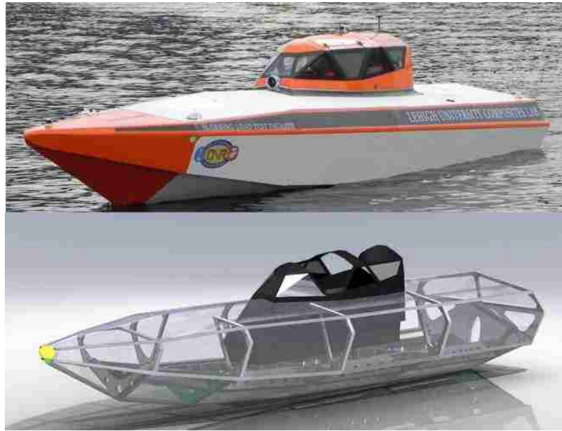
Figure 4-1: Slamming load test facility boat
