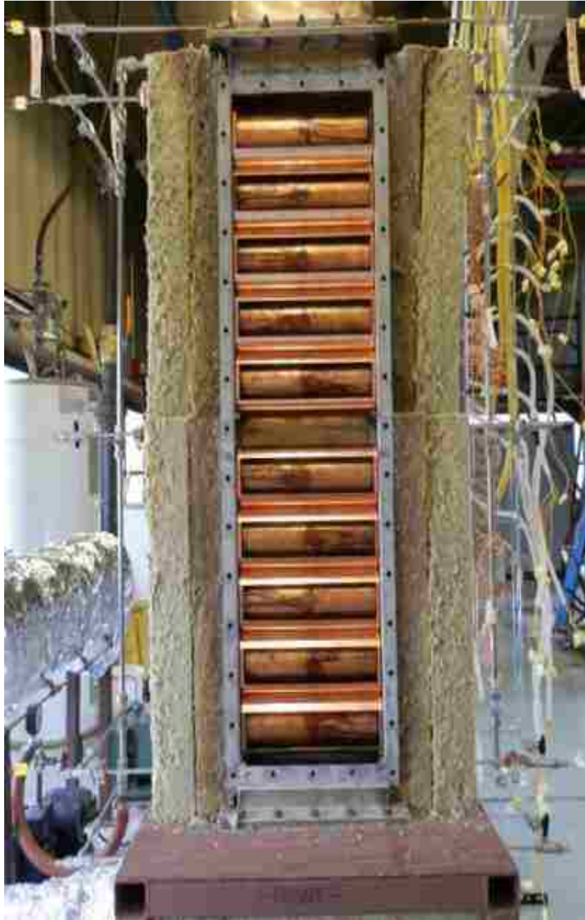
Figure 43. Thermocline model section with insulation [56, 58].
