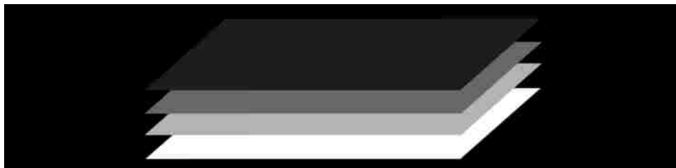
Figure 5-21 - Schematic of Section SHELL181 Element
