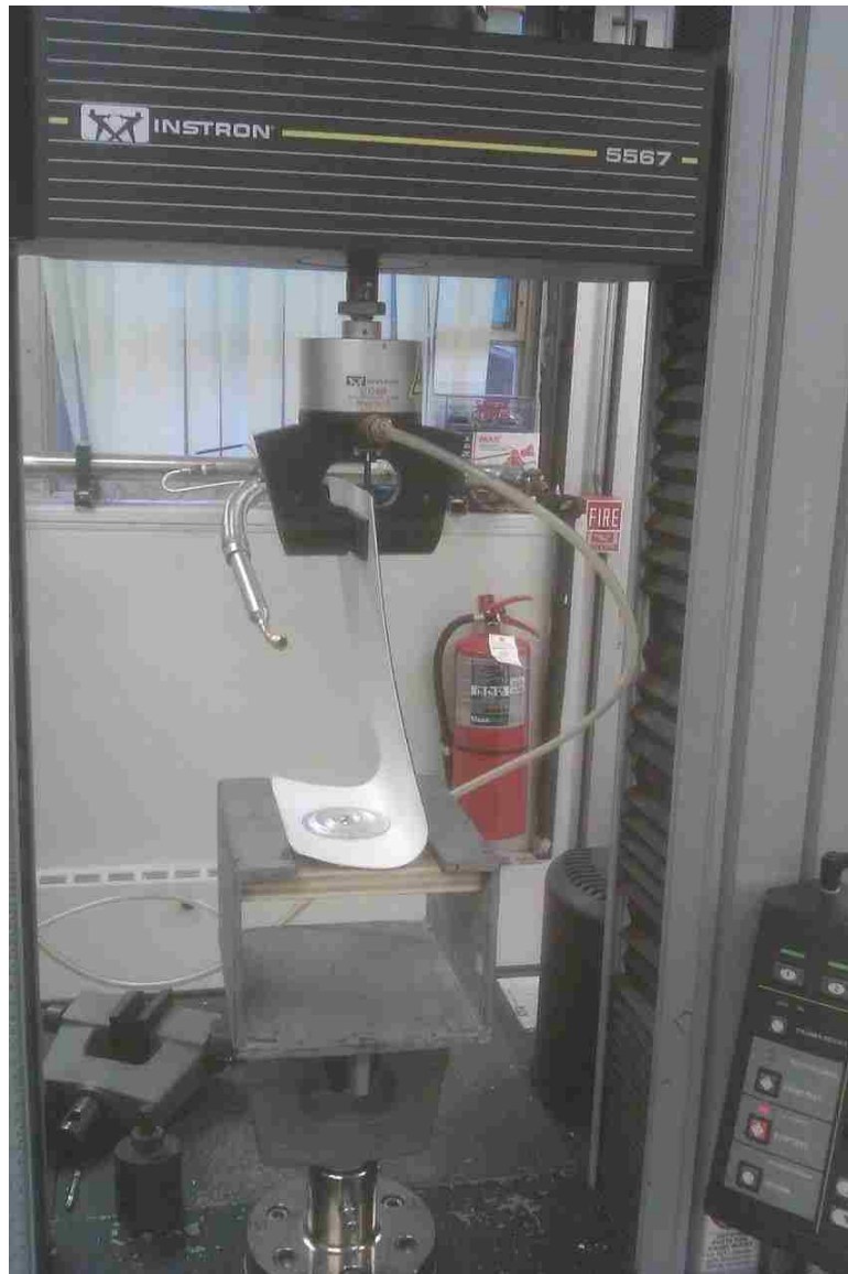
Figure 5-29- Fastener Pull-Out Test
