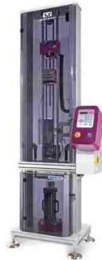
Figure 2-4 - Instron CEAST 9340 Drop Tower
