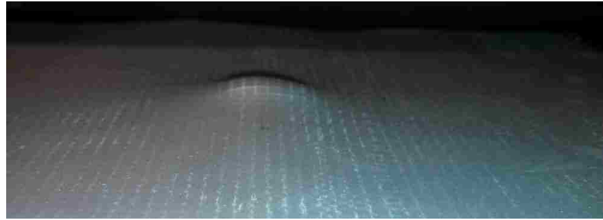
Figure 4-15 - Permanent Deflection of GAF Material
