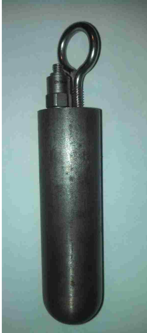
Figure 4-4 - 1" Diameter Machined Impactor
