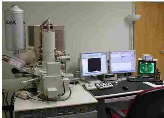
Figure 2-7. Electron Backscatter Diffraction in Scanning Electron Microscope -Hitachi 4300SE/N
