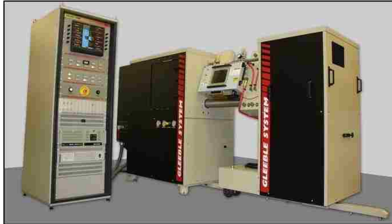
Figure 4-1. Gleeble ® 3500 System developed and manufactured by Dynamic Systems Incorporated (DSI)
