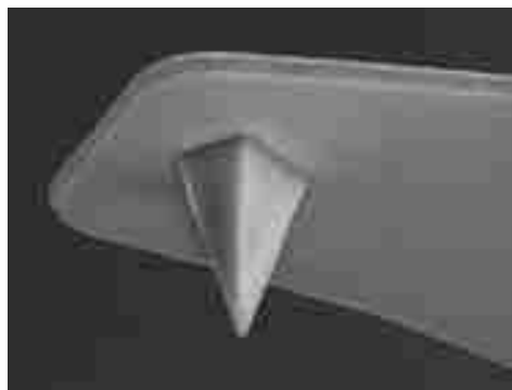
Figure 17: Silicon nitride probe used for cell indentation
