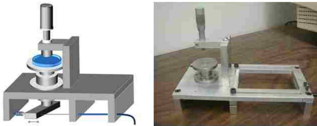
Figure 39: Remote actuated compressive loading device
