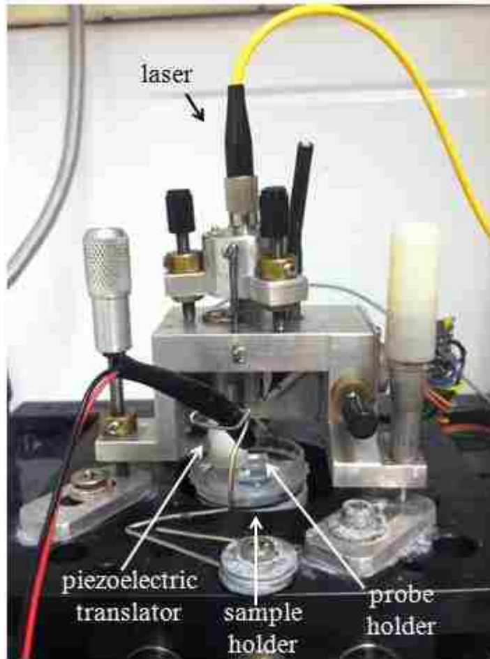
Figure 16: Home-built AFM system
