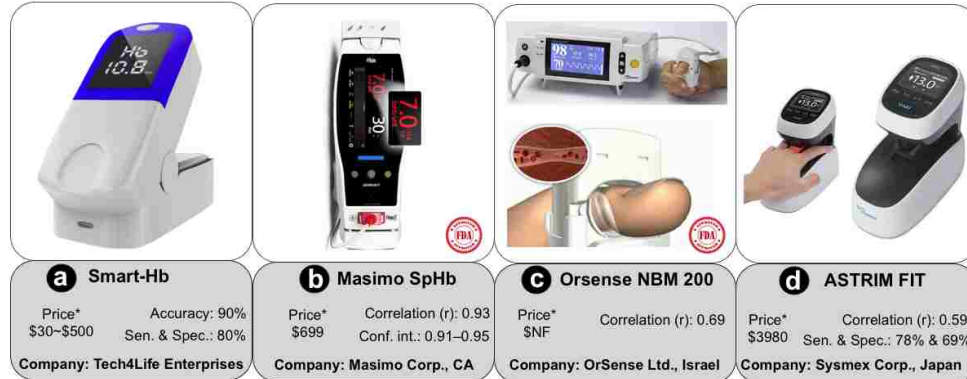
Figure 1.2: Commercial POC tools for non-invasive hemoglobin measurement. a) Smart-Hb [10], b) Masimo SpHb [11], c) NBM 200 [12], and d) Astrim-Fit [13]. The images are from respective references. *denotes the system's approximate price.
