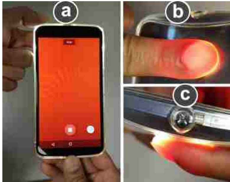
Figure 3.1: Fingertip video recording process: a) get the finger and smartphone camera ready. b) turn the built-in camera light on. c) record a video.
