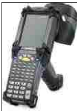
Figure 2.3 A simple RFID reader (Source: [Reader])
