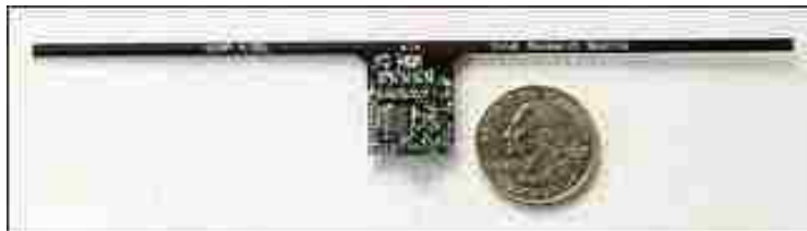
Figure 2.4 Wireless Identification and Sensing Platform (WISP) tag's size (Source: [RFID_Journal])
