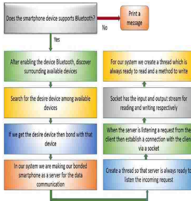
Figure 36. Algorithm on smartphone (android) for low energy communication
