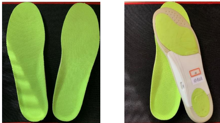
Fig [11]: Designed Insole product with embedded sensors
