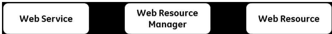
Figure 5.9: A web resource manager manages a collection of web resources. The web resource manager logically exists between the web services and a web resource.
