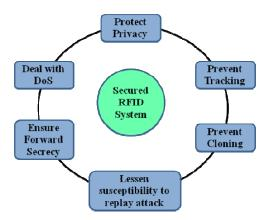
Figure 2.1: Six elements of the "Safety Ring"
