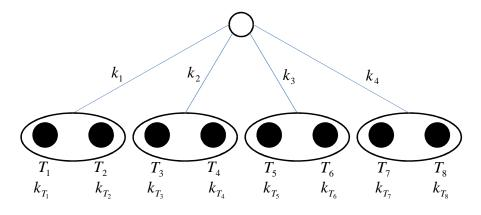
Figure 6.2: The group organization of the tags for the group based authentication protocol, with N = 8 and  $\gamma = 4$
