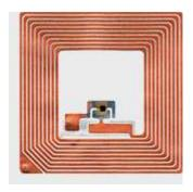
Figure 1.1: An RFID tag (source: http://www.barcode-solutions.com)
