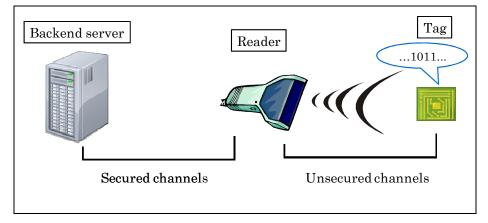
Figure 1.3: An RFID system
