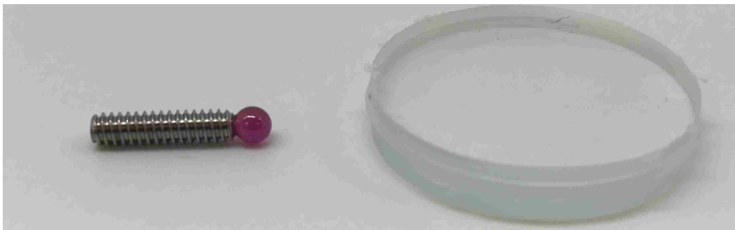
Figure 13: 3mm Ruby Probe and 25mm PDMS Sample on Glass Window
