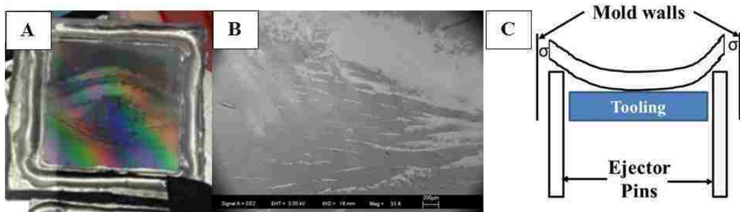
Figure 5-68: Photograph of part molded using a mold temperature of 137.8 \text{ }^{\circ}\text{C} with microfeathered and non-microfeathered regions clearly visible (A), micrograph of part displaying the same inhomogeneity (B), and schematic illustrating deflection of part responsible for inconsistent replication (C).
