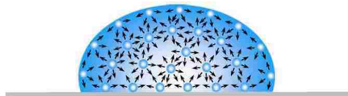
Figure 2-14: Attractive forces between water molecules in characteristic droplet [55].
