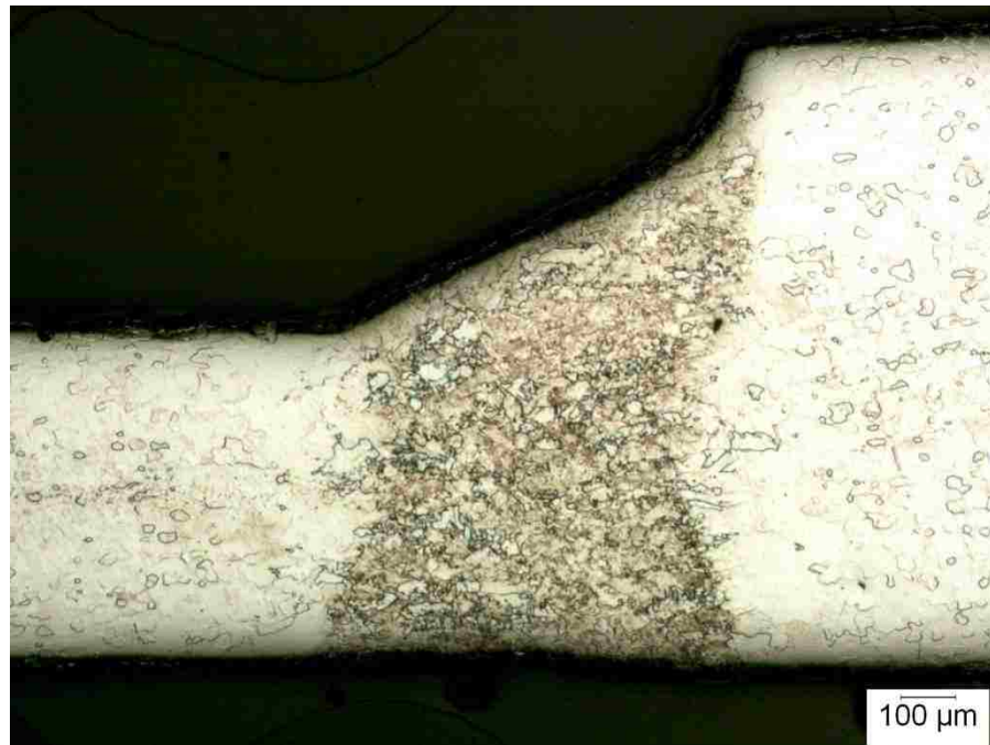
Figure 5.16 Microstructure of laser welding of BSML1
