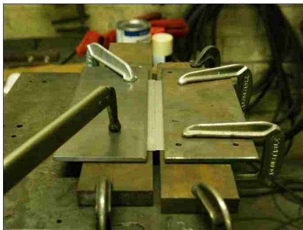
Figure 3.6 Schematic clamping situations for TIG welding experiments.
