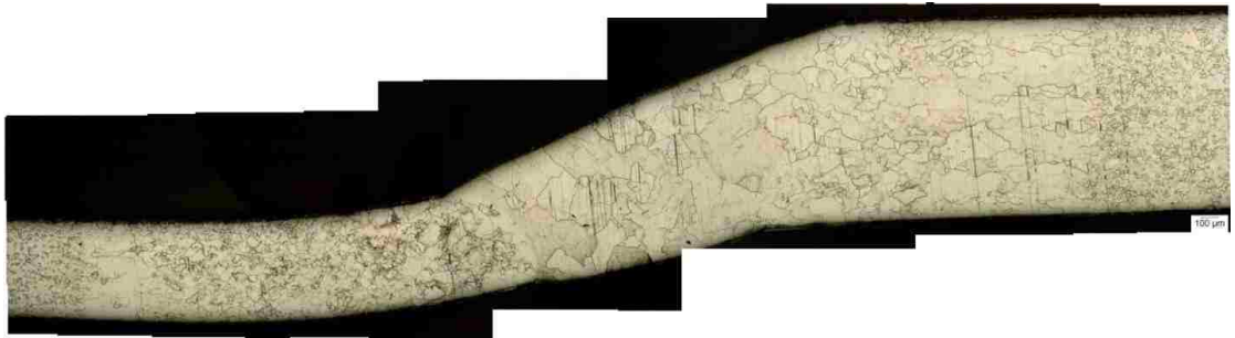
Figure 6.9 The weld pool geometry of BSMT1 in different locations.
