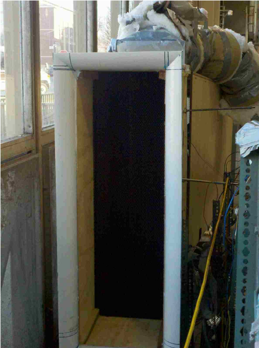
Figure 3.7 - Inlet region of the ACC showing the inlet nozzle and aluminum honeycomb.
