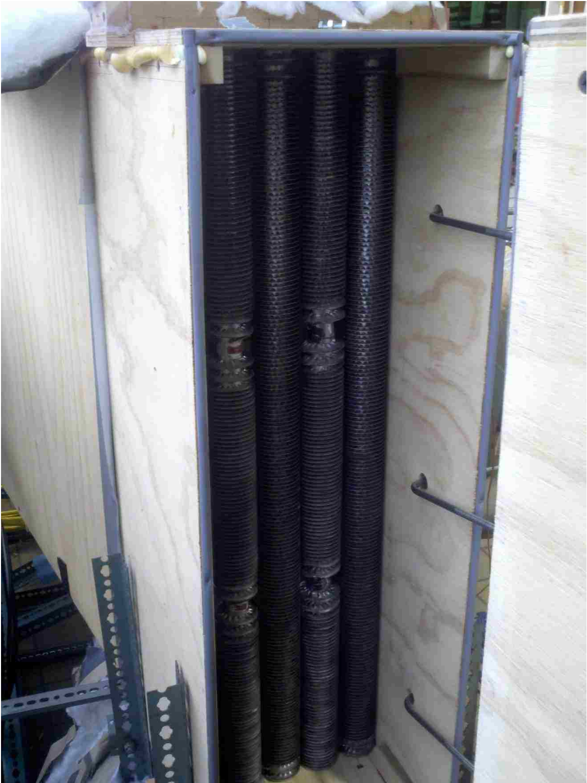
Figure 3.8 - Finned tube bundle in the main test section, along with the three pitot tubes used to measure the air-flow rate across the duct cross-section.
