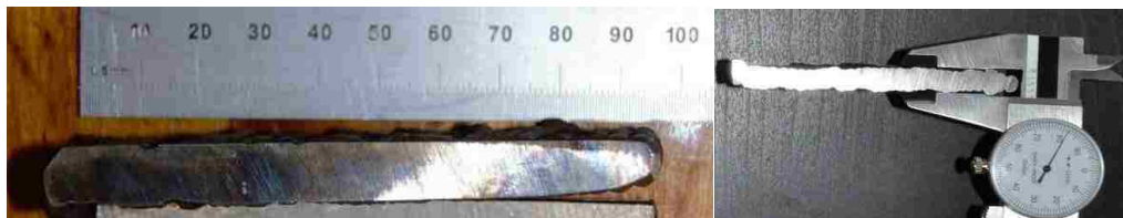
Figure 2.4 : Dimensions of the cross section (height on left and width on right)
