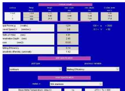
Figure 2.9 : Smart Weld screenshot shows the parameters of the welding processes
