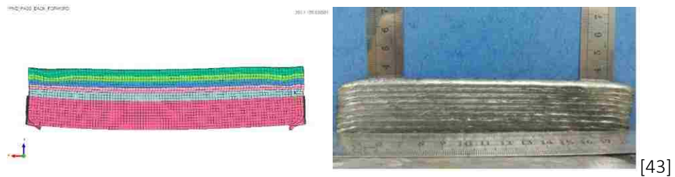
Figure 2.27 : Distortion after printing (real, bottom; simulate, top) for back forward path
