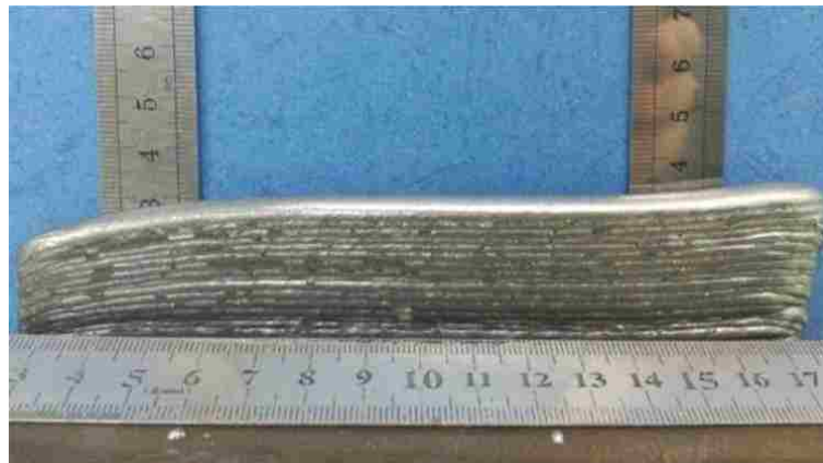
Figure 1.10 :a plate AM based, start(right) , end (left) [43]
