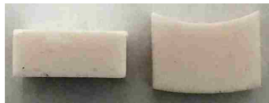
Figure 2: Left: line contact, Right: conformal contact
