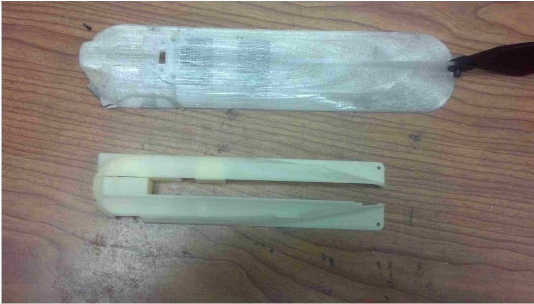
Figure C.2: A comparison between the lower fuselage of the full sized model, and the .75 scale model to be used in wind tunnel testing.
