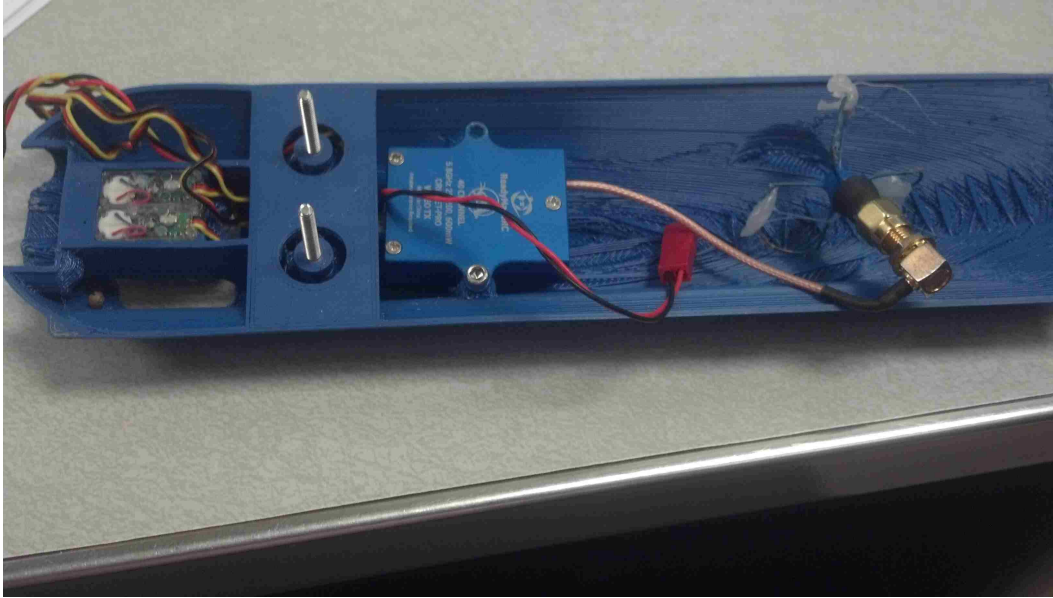
Figure 2.16: The electronics package located in the top of the Model 5 GLUAS.
