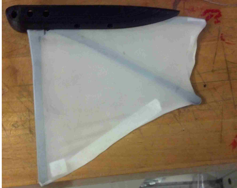
Figure 3.2: A picture of the membrane wing test model.
