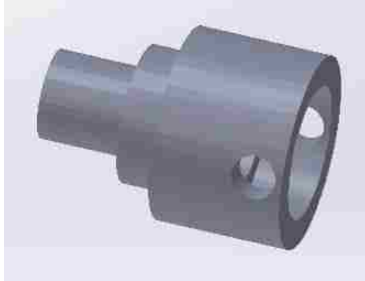
Figure 2.12: A CAD model of the propeller adapter.
