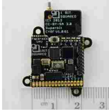
Figure 2.14: The Lisa/S autopilot board used in the GLUAS.
