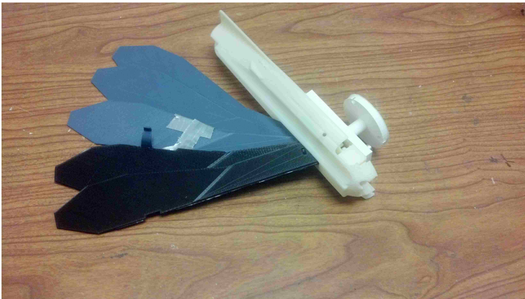
Figure C.3: The half model experimental prototype for use in wind tunnel testing.
