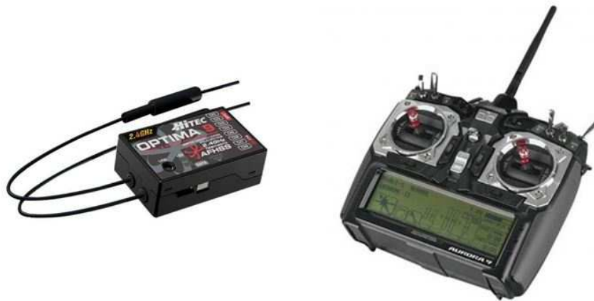
Figure 2.1: The RC receiver and the remote transmitter.
