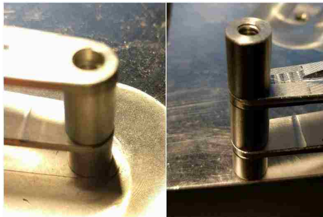
Illustration 2.1 Different combination of supports for different processing position
