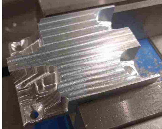
Illustration 3.2 Grab part of the blank to make room for processing slots
