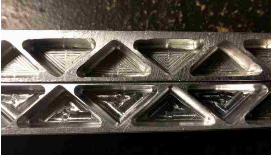
Illustration 1.3 Contrast of processed bottom (top: milled with ball mill; bottom: milled with end mill)
