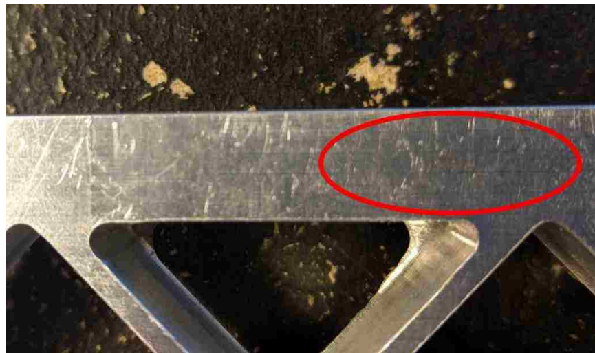
Illustration 1.1 Tool marks caused by multiple-level cutting
