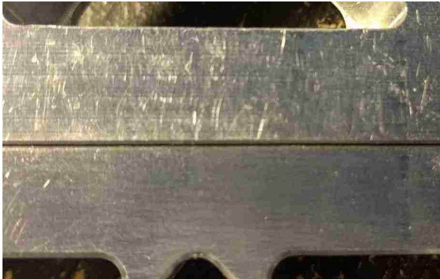
Illustration 1.2 Contrast of processed surface (top: initial trial; bottom: final part)
