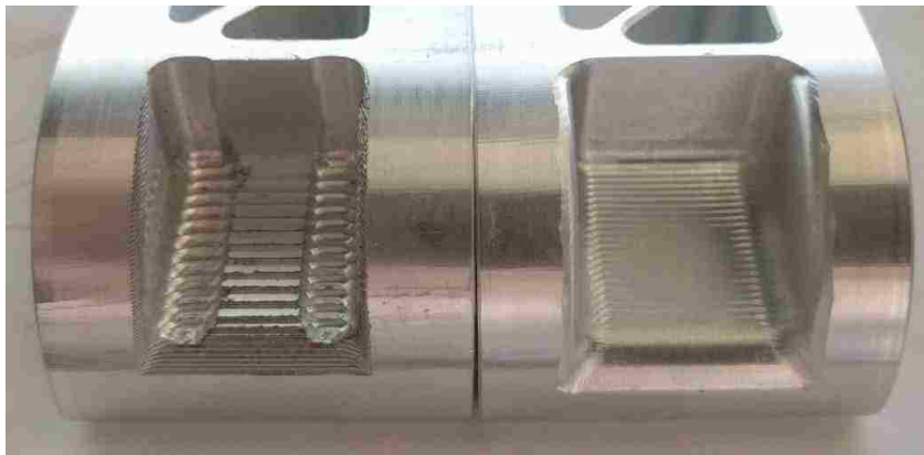
Illustration 1.4 Contrast of sloped surface processed with different step-overs
