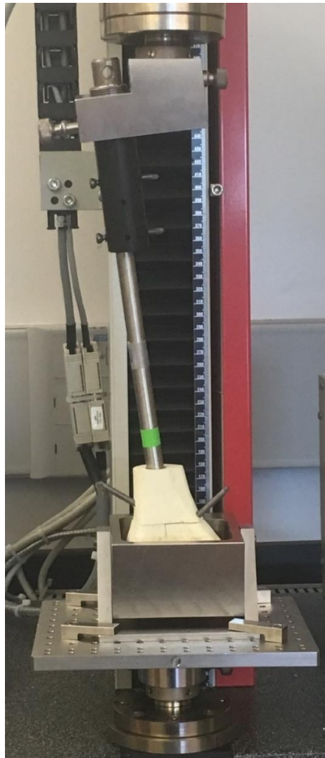
Figure 9: Test fixture for multi-axial loading with proximal mount designed for high repeatability alignment of anatomic axis
