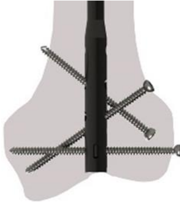
Figure 5: Representative orientation of distal locking screws. Distal locking was achieved through the use of two oblique locking screws and one transverse screw.
