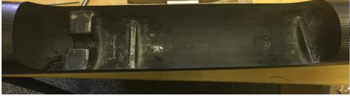
Figure 16: Bulkhead with Fiber Glass
