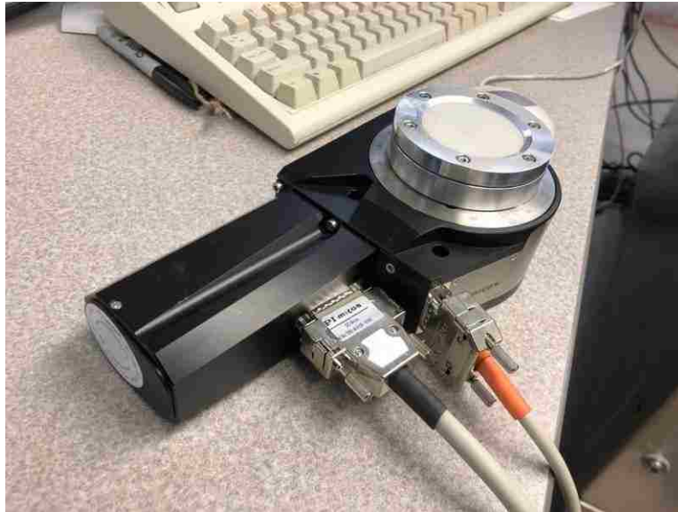
Figure 7: Pi micos rotary stage, controlled by the software to get a precise position
