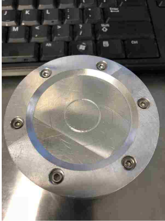
Figure 6: the outer wear scar is sliding at 100 rpm, with 1000 circles
