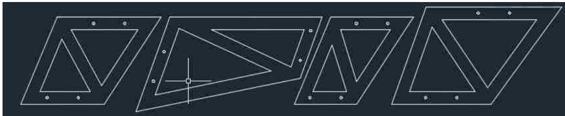
Fig 3.5 First version of linkages (from left to right: rear upper linkage, front lower linkage, rear lower linkage, front upper linkage)
