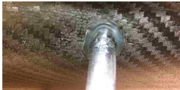
Fig 3.2 The connection between the hull and the tube
