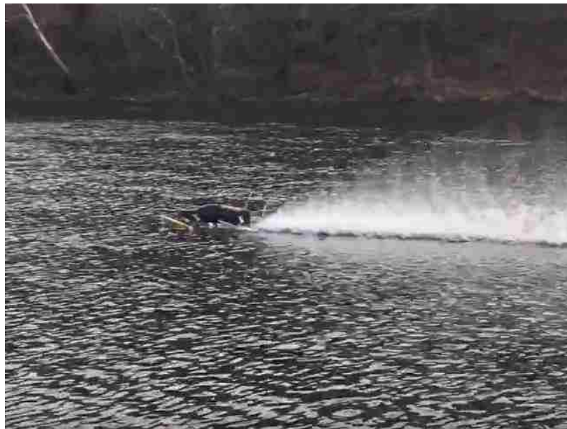
Fig 5.3 A screenshot from testing video. Note lack of spray and wake from the left front sponson.
