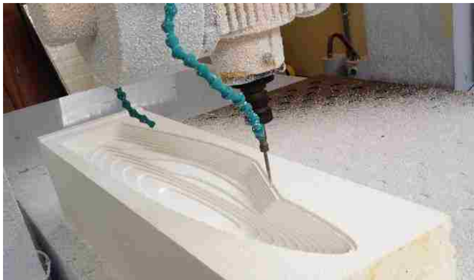
Fig 2.3 EPS mold where rough milling has been completed and finish milling has just begun.
