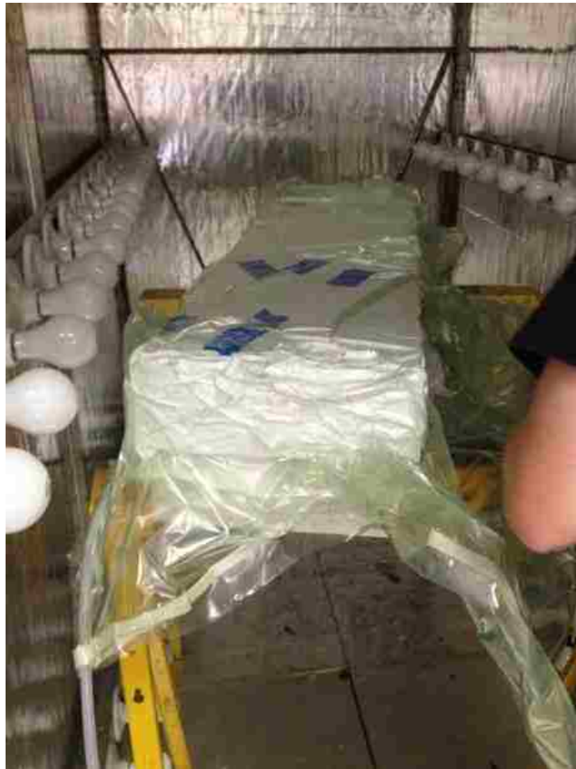
Fig 2.12 Vacuumed molds inside the oven, ready to be cured
