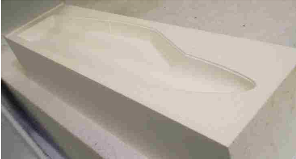
Fig 2.4 EPS mold with offset error. The error was fixed before the final molds were machined.
