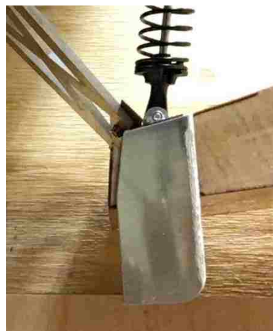
Fig 6.1 The vertical fin installed on one of the front sponsons
