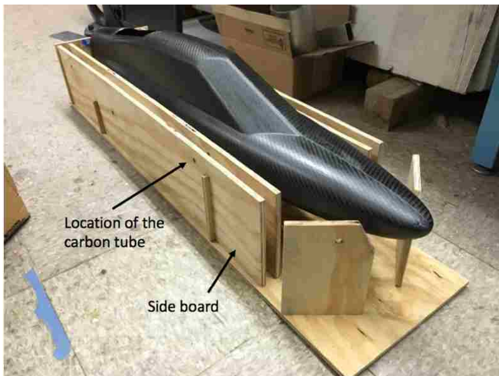
Figure 11: The jig and the hull
