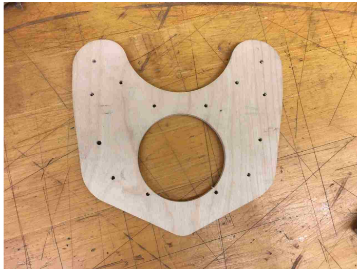
Figure 15: The wooden test sample of the motor mount
