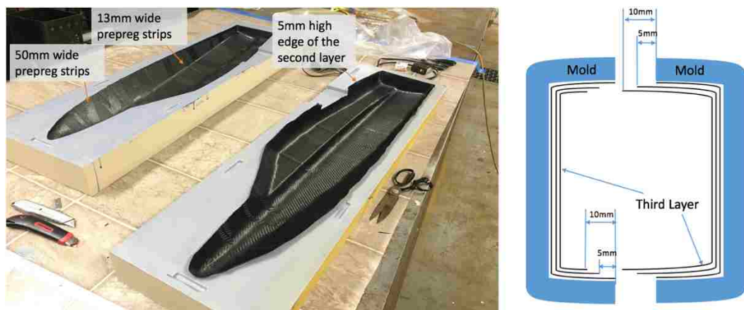
Figure 3: Hull mold (left) and sketch of overlap (right)
