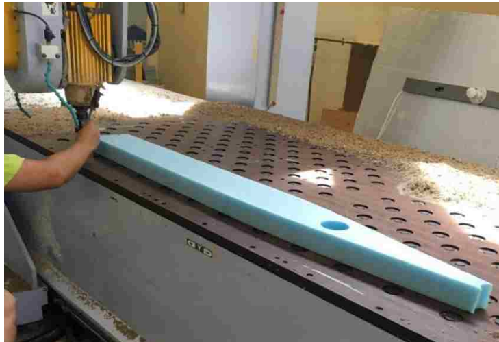
Figure 5: The foam be milled by the large 5-axis CNC router
