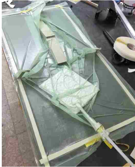
Figure 8: The setup of the vacuum bag for bonding plywood sheets on a sponson
