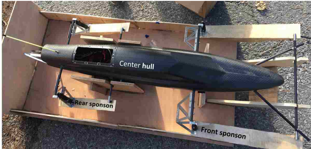
Figure 12: Top view of the suspension boat
