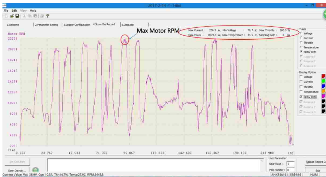
Figure 23: The Motor RPM vs Time for test 3
