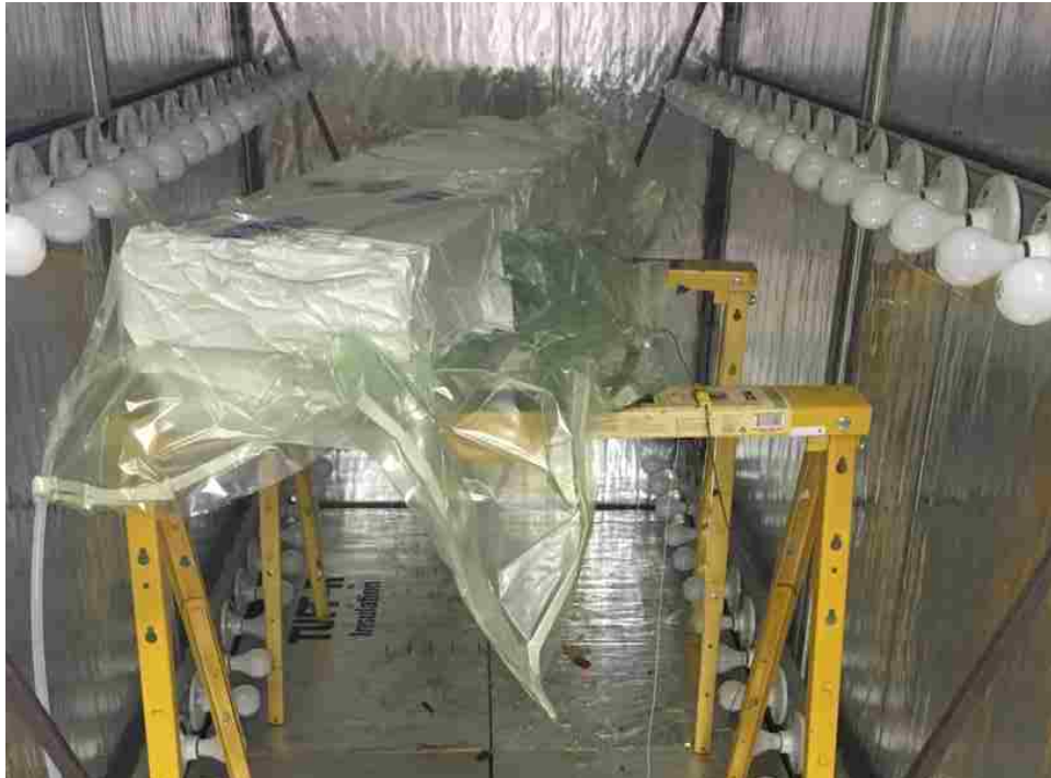
Figure 4: The mold inside an envelope bag, placed in the oven, ready to be cured
