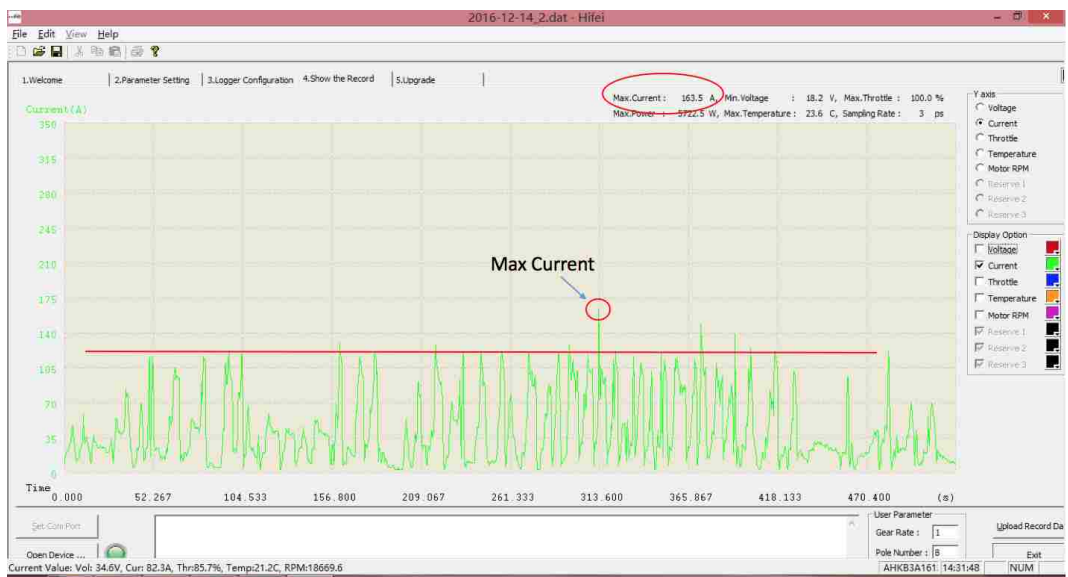
Figure 20: The Current vs Time for Test 2
