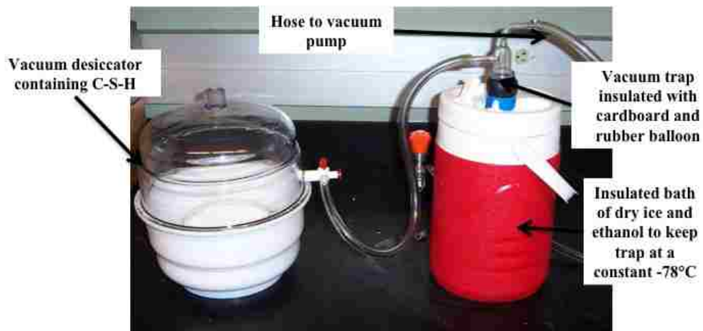
Figure 3.3: Set-up of D-drying method
