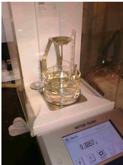
Figure 3.11: Analytical balance used for density measurements
