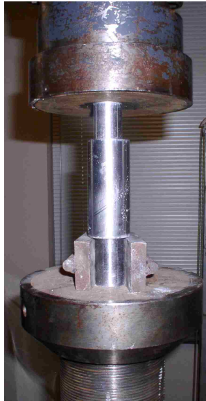
Figure 3.8: Apparatus for compacting discs of C-S-H
