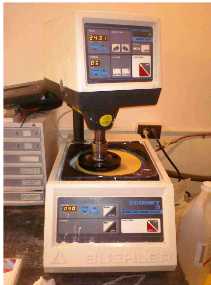
Figure 3.16: Auto-polisher used in preparation of nanoindentation specimens
