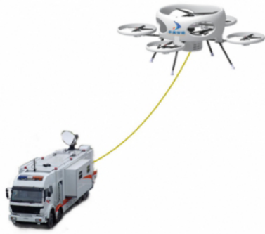
(a) An UAV tethered to a base.
