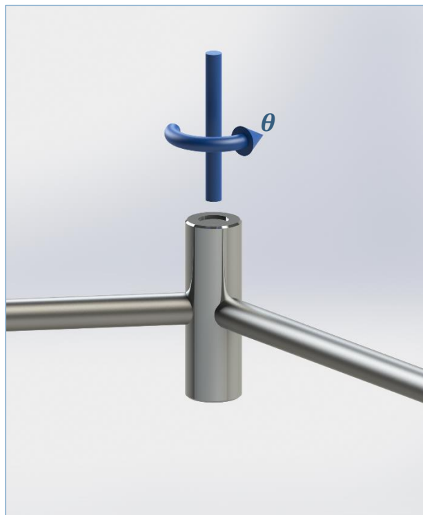
Figure 8. Diagram of the degree of freedom between two bodies permitted by a revolute joint
