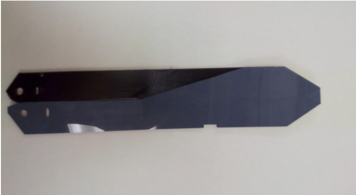
Figure 34: Overlapping wing sections for packaging
