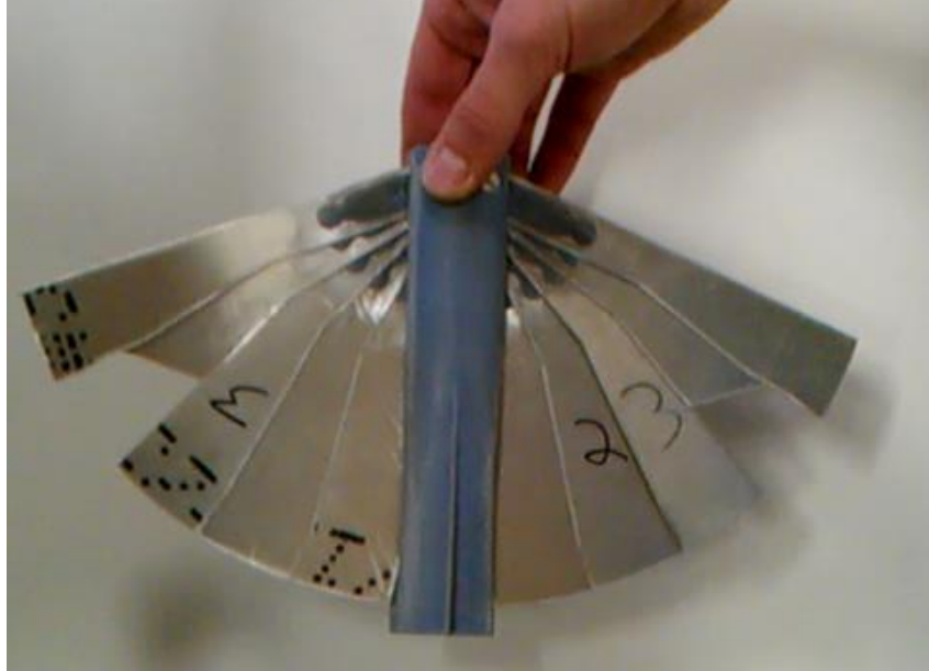
Figure 1: GLUAS Model 1 with 3D printed fuselage and aluminum wings
