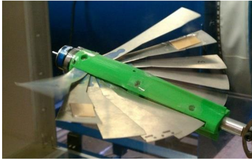
Figure 4: 40mm Model in Wind Tunnel at 10 degrees and 13.4 m/s
