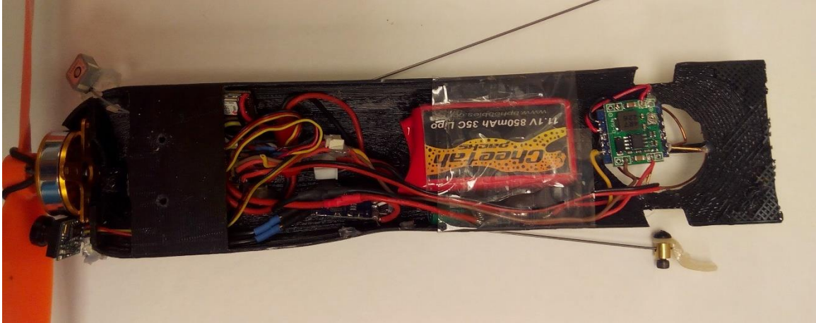
Figure 36: Packaging of video and electrical power components
