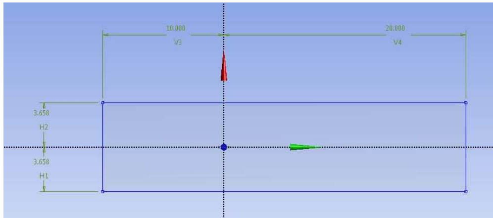
Figure 4.1: Dimensions of the computational domain. The planing plate is at the origin; it is substantially smaller than the computational domain and thus not visible in this figure.
