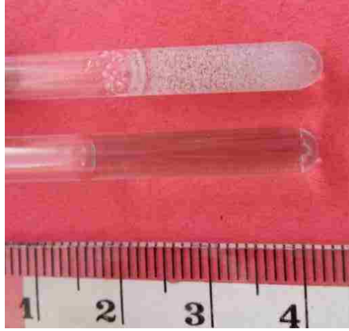
Figure 3.1: DOC/SWNT hydrogel sample: (bottom) original sample; (top) similar sample after several days upon adding terbium chloride.
