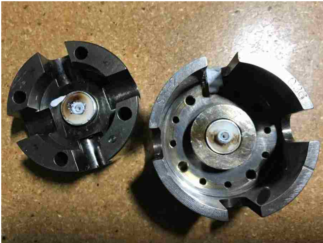
Figure 4: Diamond anvil cell with ceramic backing plates used in a resistive heating experiment.
